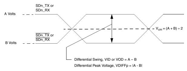
Differential Peak-Peak Voltage, VDIFFpp = 2 × VDIFFp (not shown)
