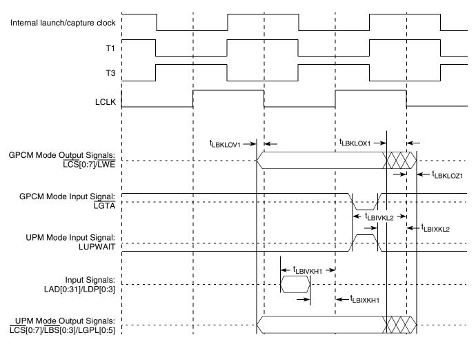
Figure 29. Local Bus Signals, GPCM/UPM Signals for LCRR[CLKDIV] = 2 (clock ratio of 4) (PLL Bypass Mode)
