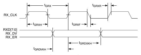
Figure 12. GMII Receive AC Timing Diagram
