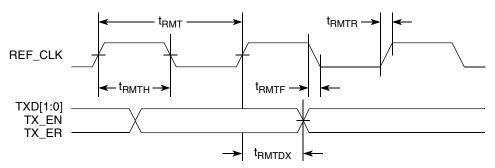
Figure 20. RMII Transmit AC Timing Diagram
