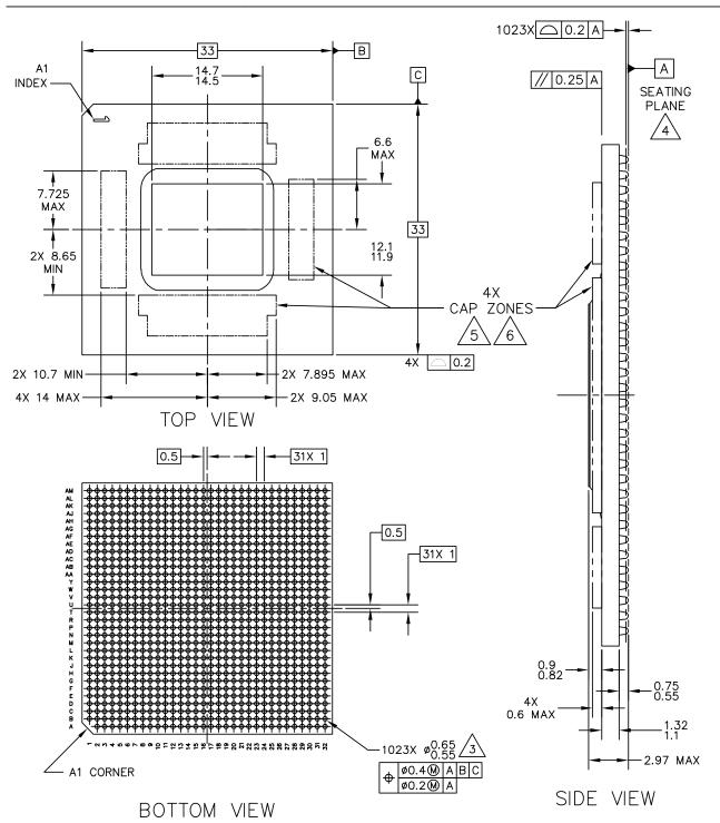
Figure 57. MPC8640D High-Lead FC-CBGA Dimensions
