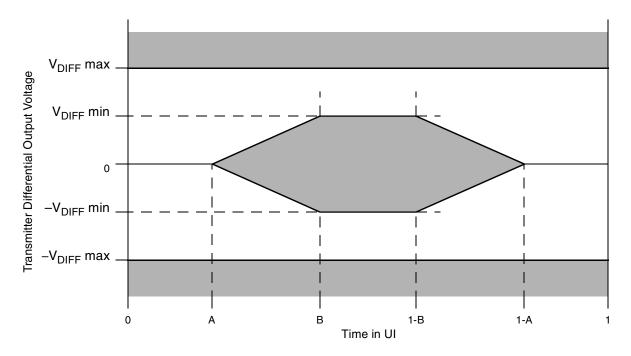
Figure 54. Transmitter Output Compliance Mask
