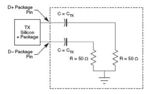
Figure 52. Compliance Test/Measurement Load
