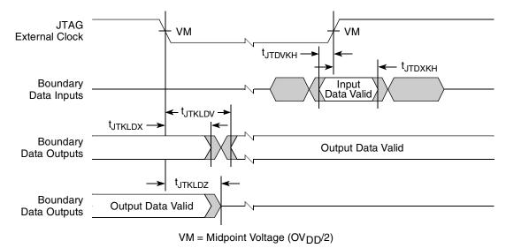
Figure 35. Boundary-Scan Timing Diagram
