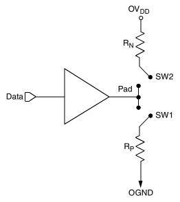
Figure 66. Driver Impedance Measurement
