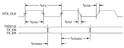
Figure 10. GMII Transmit AC Timing Diagram
