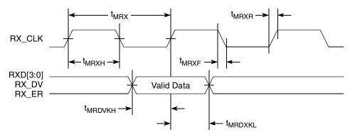
Figure 15. MII Receive AC Timing Diagram
