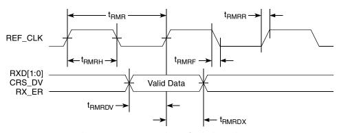
Figure 22. RMII Receive AC Timing Diagram
