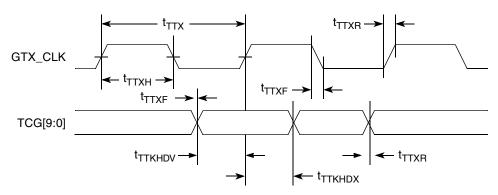
Figure 16. TBI Transmit AC Timing Diagram
