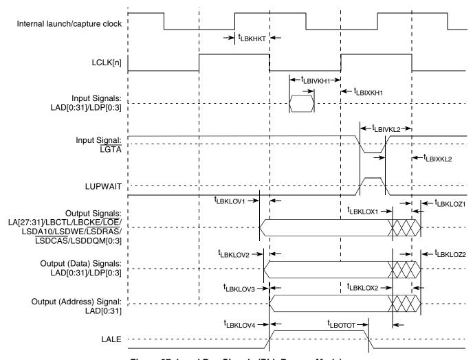
Figure 27 shows the local bus signals in PLL bypass mode.
