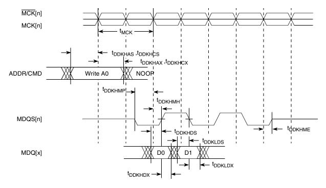
Figure 6. DDR SDRAM Output Timing Diagram
