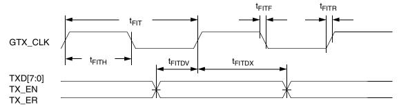
Figure 8. FIFO Transmit AC Timing Diagram
