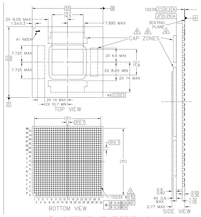
Figure 58. MPC8640D Lead-Free FC-CBGA Dimensions
