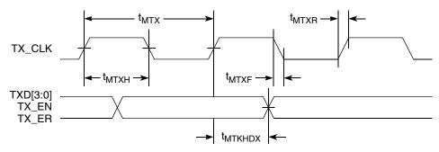
Figure 13. MII Transmit AC Timing Diagram
