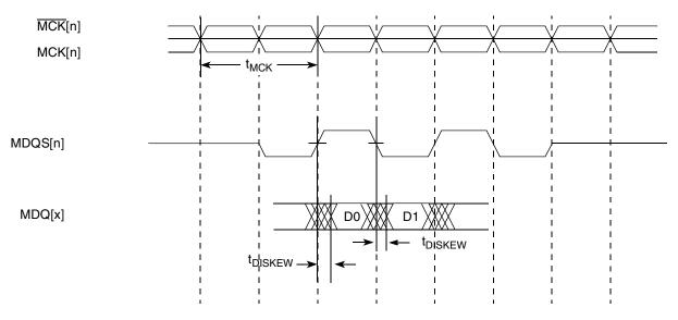
Figure 4. DDR Input Timing Diagram for tDISKEW
