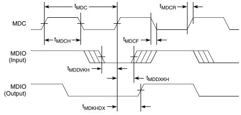
Figure 24. MII Management Interface Timing Diagram
