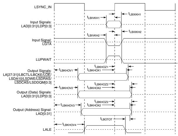
Figure 26 shows the local bus signals with PLL enabled.
