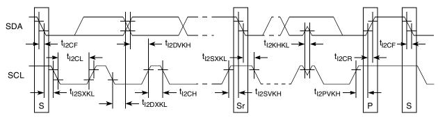
Figure 37. I<sup>2</sup>C Bus AC Timing Diagram
