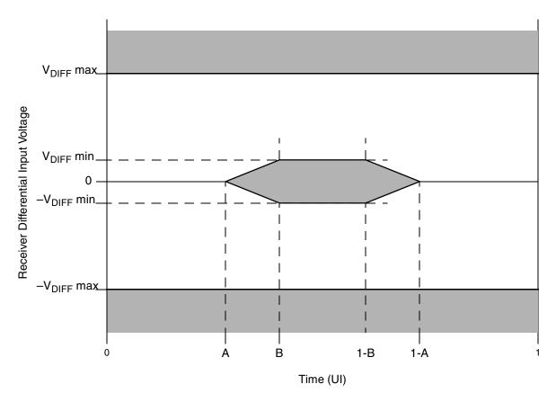
Figure 56. Receiver Input Compliance Mask
