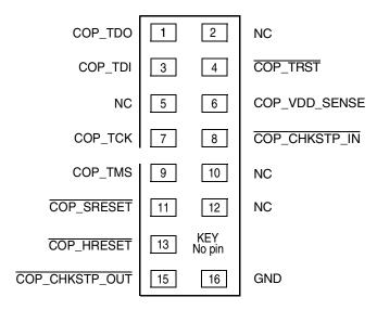
Figure 67. COP Connector Physical Pinout
