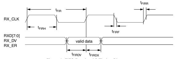
Figure 9. FIFO Receive AC Timing Diagram
