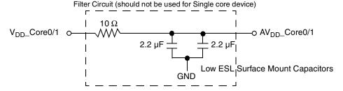
**Note:** For single core device the filter circuit (in the dashed box) should be removed and  $AV_{DD}$ \_Core1 should be tied to ground with a weak (2–10 k $\Omega$ ) pull-down resistor.
