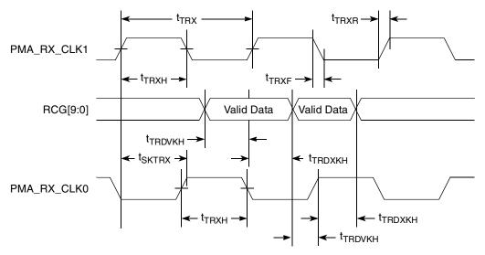
Figure 17. TBI Receive AC Timing Diagram
