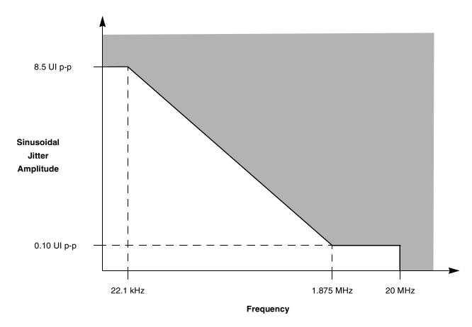
Figure 55. Single Frequency Sinusoidal Jitter Limits
