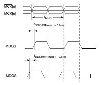
Figure 5. Timing Diagram for tDDKHMH
