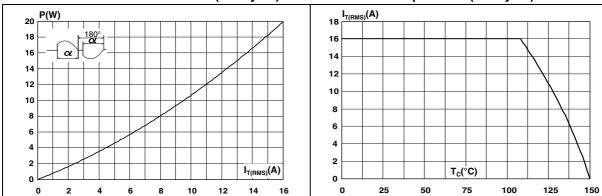
Figure 3. On-state rms current versus ambient temperature (free air convection)
