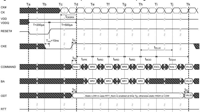
Figure 4. Reset and Initialization Sequence at Power-on Ramping
