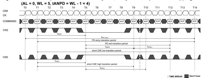
Figure 77. Power-Down Entry, Exit Clarifications-Case 1
