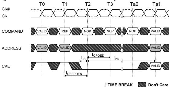
Figure 62. Active Command to Power-Down Entry
