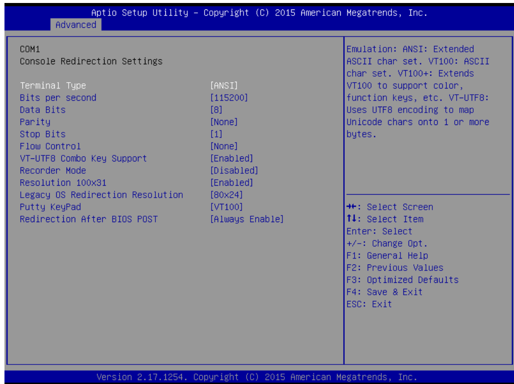
Figure 3.14 Console Redirection Setting
