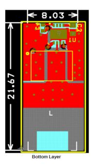
Figure 31. Recommended PCB Layout
