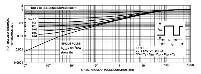
Figure 26. Junction-to-Ambient Transient Thermal Response Curve
