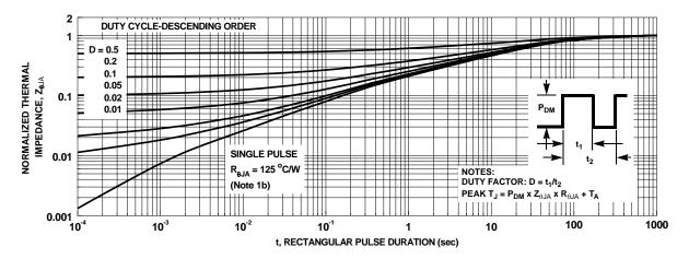
Figure 13. Junction-to-Ambient Transient Thermal Response Curve
