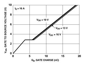
Figure 7. Gate Charge Characteristics
