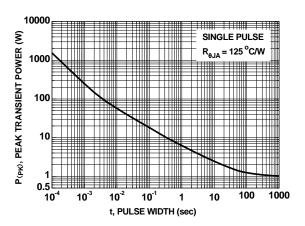
Figure 25. Single Pulse Maximum Power Dissipation
