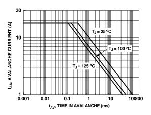
Figure 22. Unclamped Inductive Switching Capability
