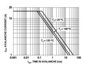
Figure 9. Unclamped Inductive Switching Capability
