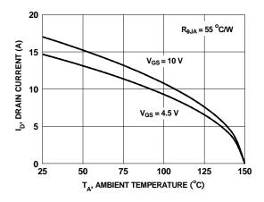
Figure 23. Maximum Continuous Drain Current vs Ambient Temperature
