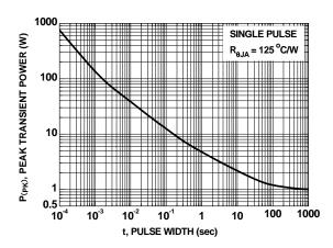
Figure 12. Single Pulse Maximum Power Dissipation
