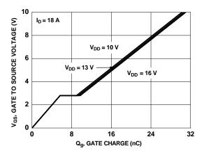
Figure 20. Gate Charge Characteristics
