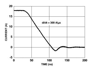
Figure 27. FDMS3616S SyncFET body diode reverse recovery characteristic
