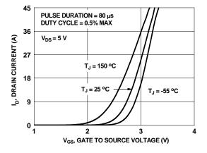
Figure 5. Transfer Characteristics
