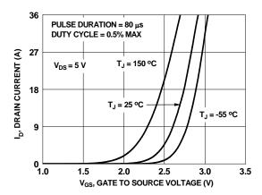
Figure 18. Transfer Characteristics
