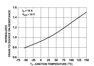
Figure 16. Normalized On-Resistance vs Junction Temperature
