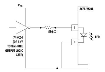
When using an open-collector TTL or open-drain CMOS logic gate, the circuit in Figure 16 can be used. When using a CMOS gate to drive the optocoupler, the circuit shown in Figure 17, where the resistor is recommended to connect to the anode of the LED, can be used.
