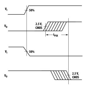
**Figure 10 Parallel Data Transmission Example**
