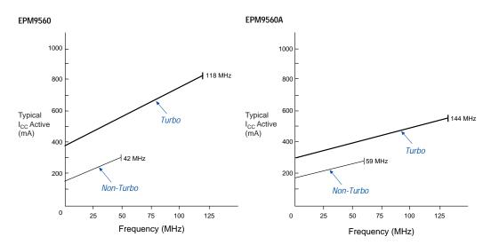
Figure 15. I<sub>CC</sub> vs. Frequency for MAX 9000 Devices (Part 2 of 2)
