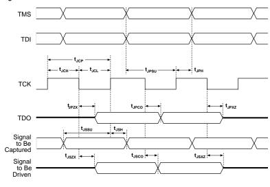
Figure 11. MAX 9000 JTAG Waveforms
