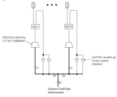
Figure 9. MAX 9000 Column-to-IOC Connections
