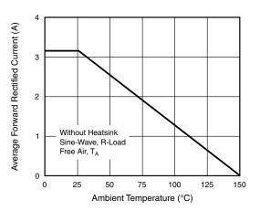
Fig. 2 - Forward Current Derating Curve
