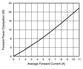
Fig. 3 - Forward Power Dissipation
