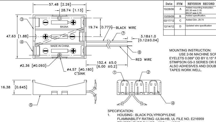
USE 2-56 MACHINE SCREWS OR EYELETS 0.089" OD BY 0.15" FLANGE STIMPSON GS-3 SERIES OR EQUIVALENT. ALSO ADHESIVES AND DOUBLE SIDED
