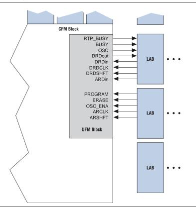
Figure 2-17. EPM570, EPM1270, and EPM2210 UFM Block LAB Row Interface
