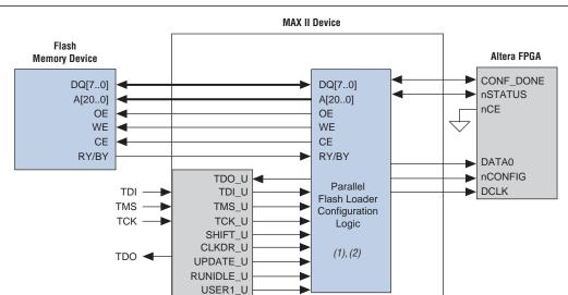
Figure 3–1. MAX II Parallel Flash Loader
