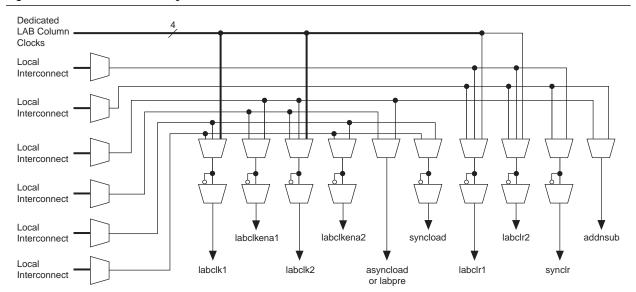
Figure 2–5. LAB-Wide Control Signals
