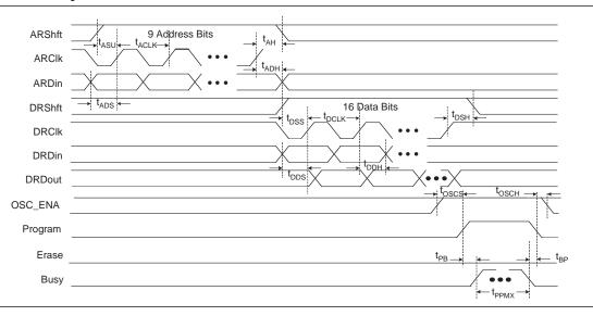
Figure 5–5. UFM Erase Waveform
