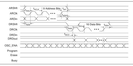
Figure 5-4. UFM Program Waveforms
