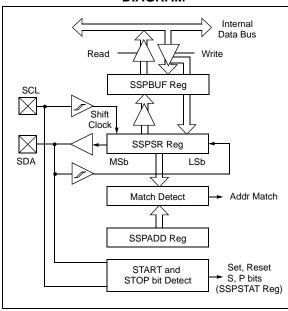
Two pins are used for data transfer. These are the SCL pin, which is the clock, and the SDA pin, which is the data. The SDA and SCL pins are automatically configured when the I<sup>2</sup>C mode is enabled. The SSP module functions are enabled by setting SSP Enable bit SSPEN (SSPCON<5>).
