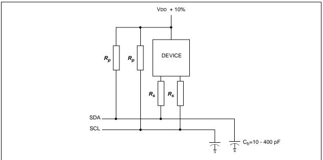
**Note:** 1<sup>2</sup>C devices with input levels related to VDD must have one common supply line to which the pull-up resistor is also connected.
