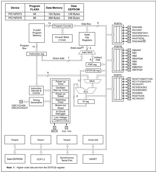
FIGURE 1-2: PIC16F874 AND PIC16F877 BLOCK DIAGRAM
