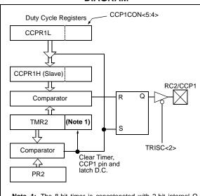
Note 1: The 8-bit timer is concatenated with 2-bit internal Q clock, or 2 bits of the prescaler, to create 10-bit time-base.
