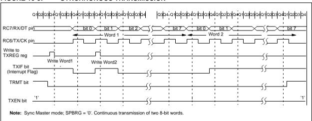
FIGURE 10-10: SYNCHRONOUS TRANSMISSION (THROUGH TXEN)
