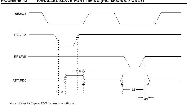
FIGURE 15-12: PARALLEL SLAVE PORT TIMING (PIC16F874/877 ONLY)
