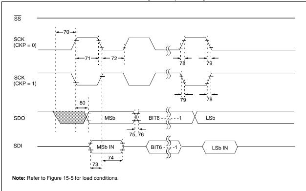
FIGURE 15-14: SPI MASTER MODE TIMING (CKE = 1, SMP = 1)
