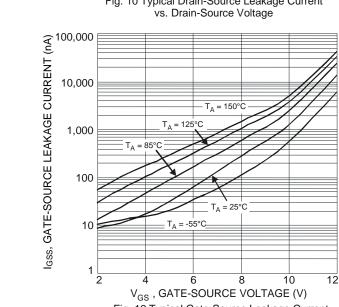
Fig. 12 Typical Gate-Source Leakage Current vs. Gate-Source Voltage
