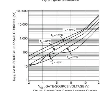
Fig. 11 Typical Gate-Source Leakage Current vs. Gate-Source Voltage
