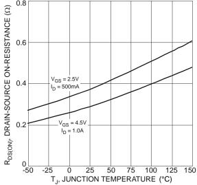
Fig. 6 On-Resistance Variation with Temperature
