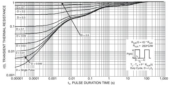
Fig. 13 Transient Thermal Response
