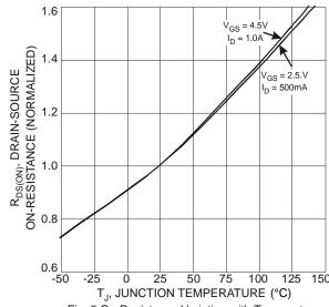
Fig. 5 On-Resistance Variation with Temperature
