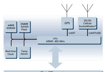
80 pin B2B connector Battery / GPIO / ADC / SPI / I2C / JTAG / Ethernet / USB Host / USB Device / GPS PPS - Data / Serial UARTs / LEDs
