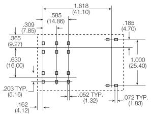
An alternate PC board layout utilizes .076  $\pm$  .003 (1.93  $\pm$  .076) diameter holes on the same center-to-center spacing shown above. Use of the rectangular holes is recommended for improved solderability.
