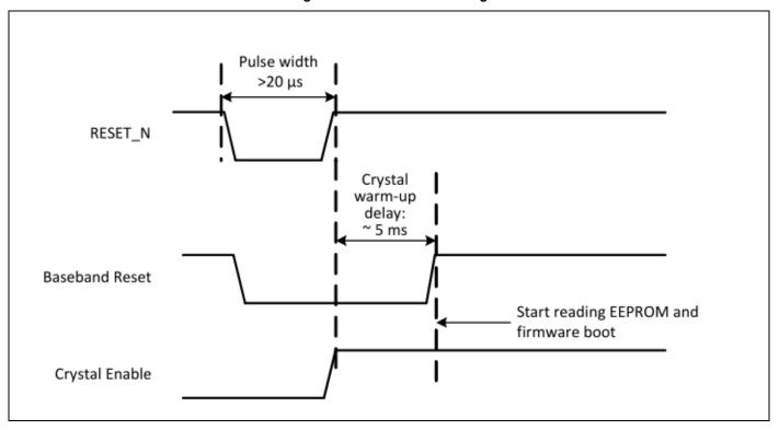
Figure 2. External Reset Timing
