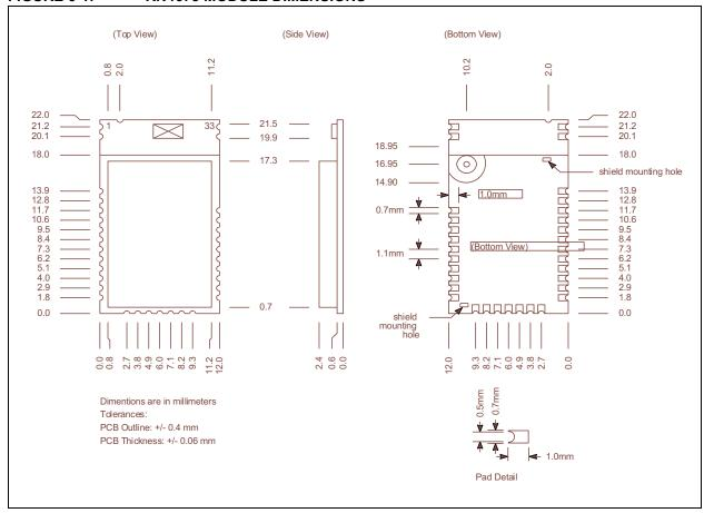
Figure 5-2 illustrates the recommended host PCB foot print.
