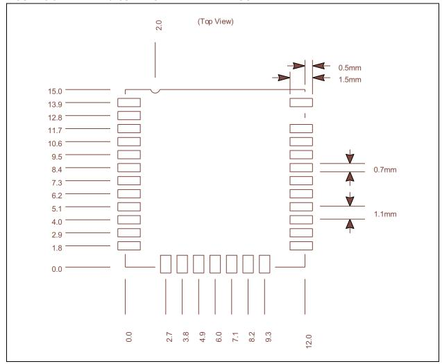
Figure 5-6 illustrates the recommended mounting details for the RN4678U module and recommended layout of the host PCB.
