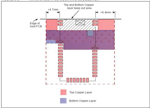
Figure 5-4 illustrates the physical dimensions of the RN4678U module.
