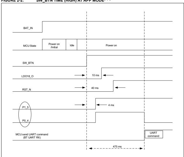
**Note 1:** Time duration (475 ms) is for reference purpose only. Use the Status Indication pins to verify the exact time when the host MCU can start sending the commands.
