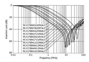
Common Mode Insertion Loss-Frequency Characteristics
