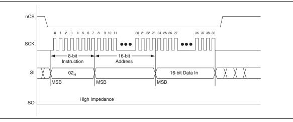
Figure 7–24 shows the WRITE operation sequence for Base mode.
