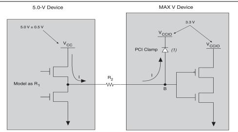
Figure 5–4. Driving a MAX V PCI-Compliant Device with a 5.0-V Device
