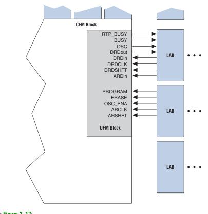
Figure 2–17. 5M240Z, 5M570Z, 5M1270Z, and 5M2210Z UFM Block LAB Row Interface (Note 1)
