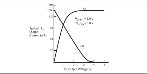
As shown in Figure 5–5,  $R_1 = 5.0 \text{ V}/135 \text{ mA}$ .
