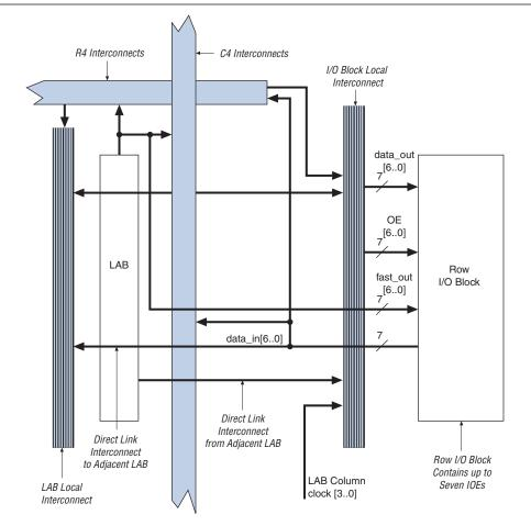
Figure 2–20. Row I/O Block Connection to the Interconnect (Note 1)
