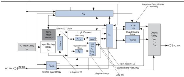
Figure 3–2. Timing Model for MAX V Devices
