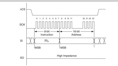
Figure 7–26 shows the SECTOR-ERASE operation sequence for Base mode.
