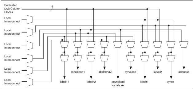
Figure 2–5. LAB-Wide Control Signals
