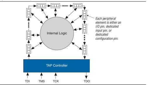
Figure 8–3. Boundary-Scan Register
