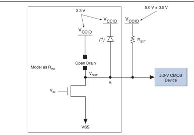
Figure 5-3. MAX V Device Compatibility with 5.0-V CMOS Devices
