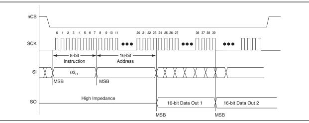
Figure 7–22 shows the READ operation sequence for Base mode.
