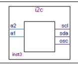
ALTUFM\_I2C megafunction is under the **Memory Compiler** folder on page 2a of the MegaWizard Plug-In Manager. On page 3, you can choose whether to implement the **Read/Write** or **Read Only** mode for the UFM. You also have an option to choose the memory size for the ALTUFM\_I2C megafunction as well as defining the four MSBs of the slave address (default 1010).
