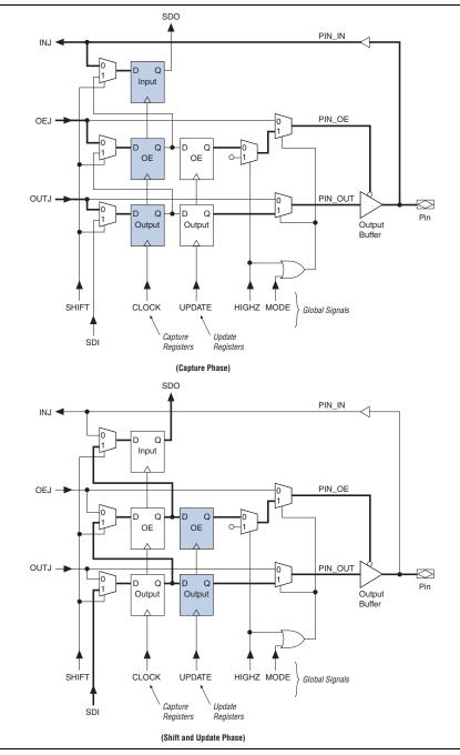
Figure 8–11 resembles the SAMPLE/PRELOAD waveform diagram, except that the instruction code for EXTEST is different. The data shifted out of TDO consists of the data that was present in the capture registers after the capture phase. New test data shifted into the TDI pin appears at the TDO pin after being clocked through the entire boundary-scan register.
