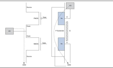
When the I/O pin receives a negative ESD zap at the pin that is less than -0.7 V (0.7 V is the voltage drop across a diode), the intrinsic
