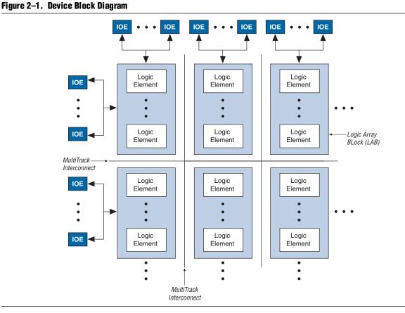
Figure 2-1 shows a functional block diagram of the MAX V device.
