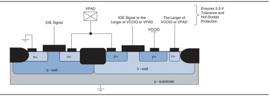
The CMOS output drivers in the I/O pins intrinsically provide electrostatic discharge (ESD) protection. There are two cases to consider for ESD voltage strikes—positive voltage zap and negative voltage zap.
