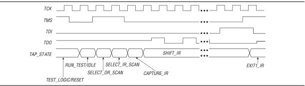
The TDO pin is tri-stated in all states except the SHIFT\_IR and SHIFT\_DR states. The TDO pin is activated at the first falling edge of TCK after entering either of the shift states and is tri-stated at the first falling edge of TCK after leaving either of the shift states.
