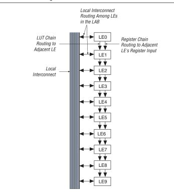
Figure 2–11. LUT Chain and Register Chain Interconnects
