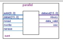
ALTUFM\_PARALLEL megafunction is under the **Memory Compiler** folder on page 2a of the MegaWizard Plug-In Manager. On page 3, you can choose whether to implement the **Read/Write** or **Read Only** mode for the UFM. You also have an option to choose the width for address bus (up to 9 bits) and for the data bus (up to 16 bits). You can specify the initial content of the UFM block on page 4 of the ALTUFM MegaWizard Plug-In Manager as discussed in "Creating Memory Content File" on page 7–39.
