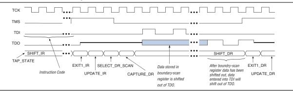
Figure 8–11. EXTEST Shift Data Register Waveforms
