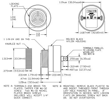
NOTE B: MOUNTING- REMOVE BLACK PLASTIC NUT AND INSERT THREADED FRONT THROUGH 1.25' HOLE PUNCHED IN PANEL, IF DRIENTATION IS NEEDED, NOTE LOCKING FLATS ON DRAVING, SCREW NUT BACK ON. DO NOT OVERTIGHTEN.
