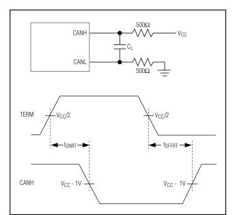
Figure 4. Test Circuit and Diagram for TERM Timing (MAX3059)
