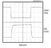
**DRIVER PROPAGATION DELAY (RS = GND)**
