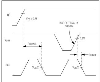
Figure 2. Timing Diagram for Standby Signal (MAX3058)
