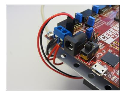
MPLAB or MPIDE can now be used to program the *MotorRobot* demo project to the board. Again, this demo project can be downloaded from the Motor Robot Kit product page at digilentinc.com. Note that running the reference design requires that the power select mode jumper J12 be shorted to External Power (EXT). Once the board has been programmed with the reference design, pressing BTN2 will cause the motors to turn while pressing BTN1 will cause them to stop.
