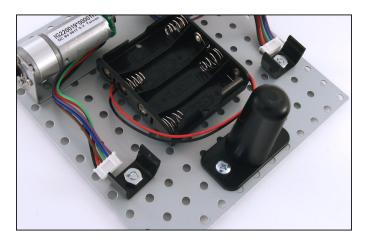
6. Attach the two PmodHB5 modules to the Pmod clips and connect them to the motors.
