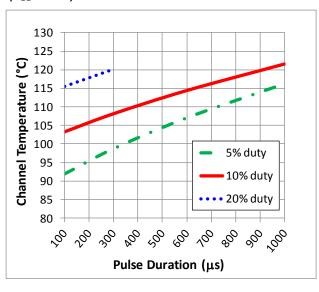
Max. Transient Channel Temp. vs. Pulse Width  $(V_{DD} = 45 \text{ V})$
