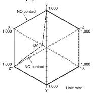
Sample: G2RL-14 12 VDC Number of Relays: 5 pcs Test conditions: Shock is applied in ±X, ±Y, and ±Z directions three times each with without energizing the Relays to check the number of malfunctions.
