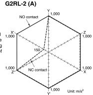
Sample: G2RL-24 12 VDC Number of Relays: 5 pcs Test conditions: Shock is applied in ±X, ±Y, and ±Z directions three times each with without energizing the Relays to check the number of malfunctions.
