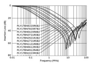
Common Mode Insertion Loss-Frequency Characteristics
