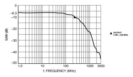
Figure 2. Typical EMI Filter Response (50  $\Omega$  Source and 50  $\Omega$  Lead Termination)
