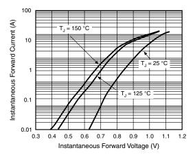
Figure 3. Typical Forward Characteristics Per Diode
