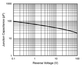
Figure 5. Typical Junction Capacitance Per Diode
