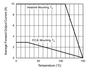
Figure 1. Derating Curve Output Rectified Current
