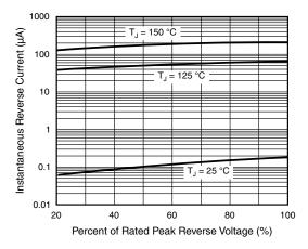
Figure 4. Typical Reverse Characteristics Per Diode
