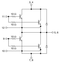
Fig. 10 - Electrical Diagram
