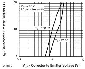
Fig. 1 - Typical Output Characteristics
