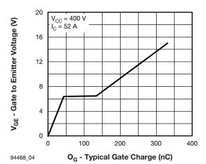
Fig. 4 - Typical Gate Charge vs. Gate to Emitter Votlage
