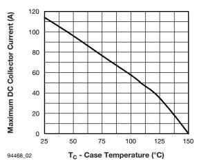
Fig. 2 - Maximum Collector Current vs. Case Temperature
