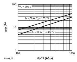
Fig. 7 - Typical Reverse Recovery Current vs. dl<sub>F</sub>/dt
