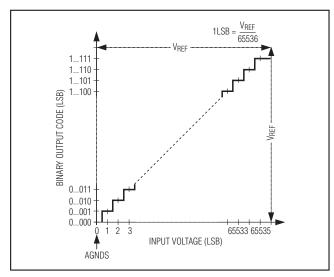
Figure 14. Unipolar Transfer Function
