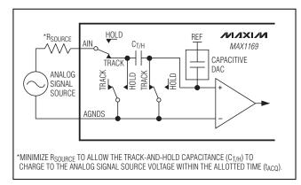
Figure 5. Equivalent Input Circuit
