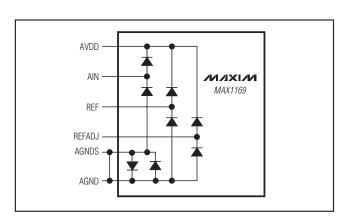
Figure 6. Internal Protection Diodes
