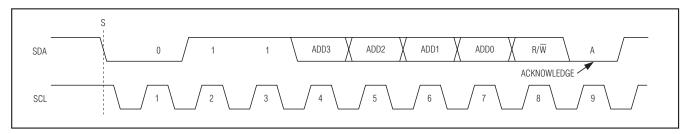
Figure 9. MAX1169 Slave Address Byte
