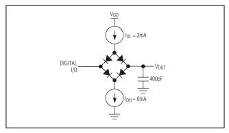
Figure 2. Load Circuit
