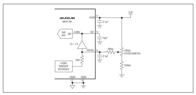
Figure 13. Adjusting the Internal Reference
