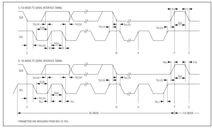
Figure 1. I<sup>2</sup>C Serial Interface Timing
