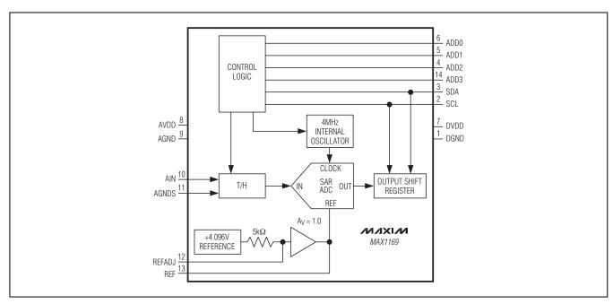
Figure 3. MAX1169 Simplified Functional Diagram
