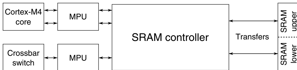
Figure 3-26. SRAM controller configuration
