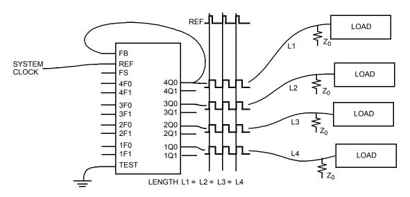
Figure 4 shows the PSCB configured as a zero skew clock buffer. In this mode the 7B991/992 is used as the basis for a low-skew clock distribution tree. When all of the function select inputs (× F0, × F1) are left open, the outputs are aligned and each drives a terminated transmission line to an independent load.
