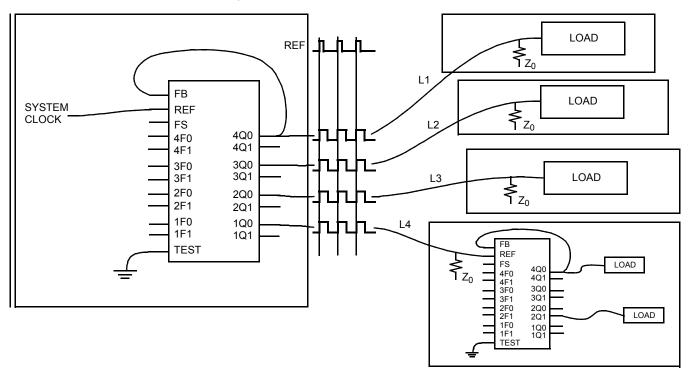
Figure 10. Board-to-Board Clock Distribution
