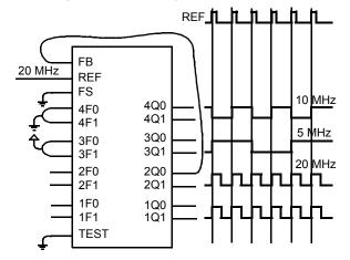
Figure 8 demonstrates the PSCB in a clock divider application. 2Q0 is fed back to the FB input and programmed for zero skew. 3Qx is programmed to divide by four. 4Qx is programmed to divide by two. Note that the falling edges of the 4Qx and 3Qx outputs are aligned. This enables the use of rising edges of the  $\frac{1}{2}$  frequency and  $\frac{1}{4}$  frequency without concern for skew mismatch. The 1Qx outputs are programmed to zero skew and
