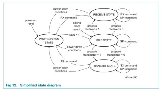
An important implication of this is that a TX operation is immediately aborted if the active mode is switched to anything except TX mode, for example, switching the device into RX mode immediately shuts down the power amplifier without smoothly ramping down the RF power.
