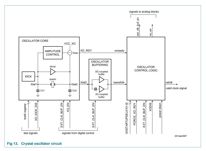
The crystal oscillator consists of three main blocks: the oscillator core, the oscillator buffer and the oscillator control logic.
