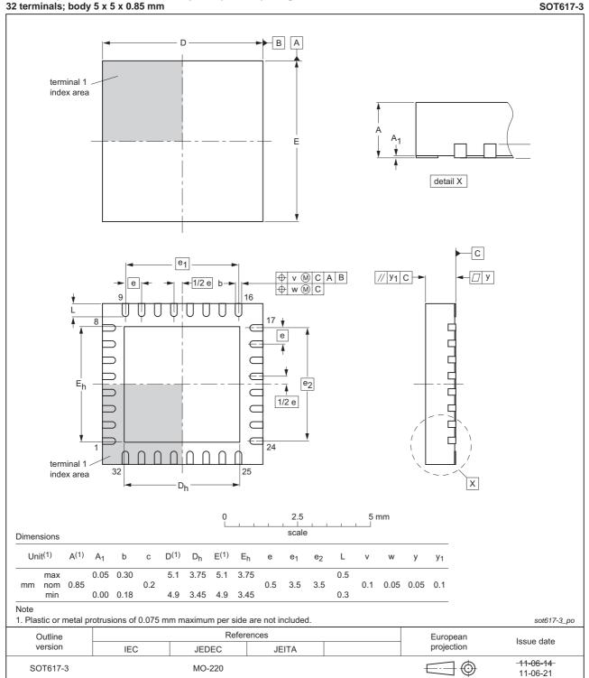
HVQFN32: plastic thermal enhanced very thin quad flat package; no leads; 32 terminals; body 5 x 5 x 0.85 mm
