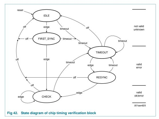
After the first synchronization (reception of two edges) the chip timing verification block becomes VALID and the chip timing CHECK begins. The last chip timing step is directly used as the ERROR criteria when in this state.
