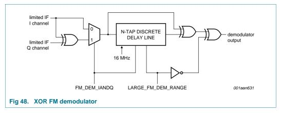
If bit FM\_DEM\_IANDQ is set to logic 0, only the limited I channel IF input is used for demodulation. In this case the demodulator is set to a center frequency of 300 kHz. If bit FM\_DEM\_IANDQ is set to logic 1, the I and the Q signals, which have a phase difference of 90 °, are combined with an XOR gate. In these circumstances the demodulator is set to a center frequency of 600 kHz as the I and Q combination effectively doubles the frequency.
