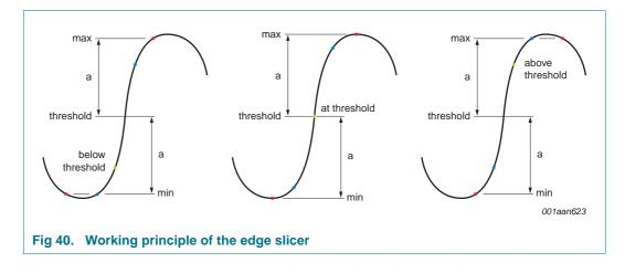
The slicer operating mode slicer is selected by the slicer selection bits SLICERSEL\_W[1:0]; see <u>Table 84 "SLICERSEL\_W bit functions</u>" on page 112.
