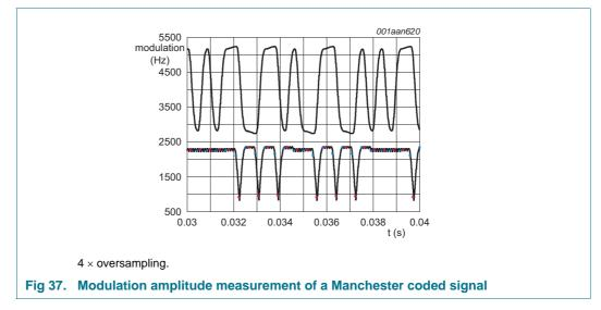
Figure 37 shows an example of the amplitude measurement when measuring a noise-free Manchester encoded baseband signal. The top waveform is the baseband signal. Note that this signal can have an arbitrary offset. The lower waveform shows the output of the amplitude measurement. The red dots show the actual values (oversampling rate of 4 versus the chip-clock) used for computation.
