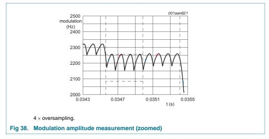
In this example the upper horizontal dashed line corresponds to the actual amplitude  $A_{act}$ . The lower horizontal dashed line corresponds to  $A_{act} - 8 \% = 0.92 A_{act}$ . Consider this when calculating the lower and upper limit for the modulation amplitude detection. The higher limit can be set close to the expected value, the lower limit must be at least 8 % lower than the expected value.
