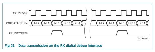
RXD\_DBG\_SEL[3:0] determines which 16-bit signal vector is sampled in parallel at 1 Msamples/s and output as a serial data stream as shown in <u>Figure 52</u>. The available debug signal vectors are given in <u>Table 27</u>.
