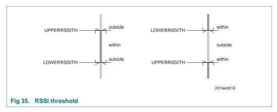
If a single minimum threshold is desired, the UPPERRSSITH[7:0] value must be set to 255 (FFh). To achieve a single maximum threshold, the LOWERRSSITH[7:0] register must be set to logic 0.
