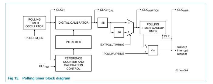
The polling timer employs a digital calibration with a modulo counter. The crystal oscillator clock  $CLK_{REF}$  is used as a reference clock for the calibration. The calibration procedure measures one period of the polling timer clock  $CLK_{PT}$  and determines the appropriate calibration value for the modulo counter. The output clock  $CLK_{PTCAL}$  has a nominal period of 62.5  $\mu$ s.
