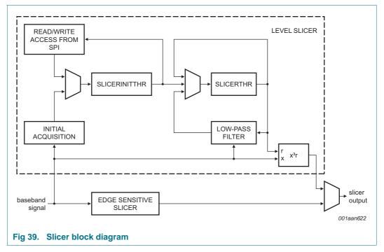
The edge-sensitive slicer will not make use of these two registers. The EDGE\_MODAMP\_TH contains the expected peak modulation amplitude with which the edge slicer is initialized. The expected peak modulation value is provided by the EDGE\_MODAMP\_TH[7:0] register; see <u>Section 8.2.1.32 "Register EMODAMPTH" on page 111</u>. The EDGE\_MODAMP\_TH is calculated by:
