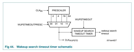
The wakeup search timer consists of a prescaler and a timer register. The clock is derived from the mainscaler clock and is therefore associated with the selected baud rate.
