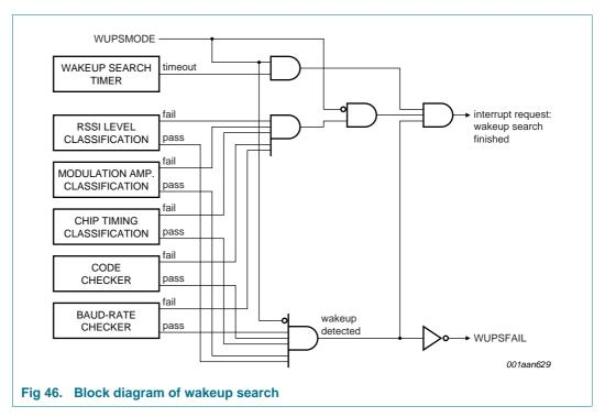
At the end of the wakeup search an interrupt request is generated and the result is stored in bit WUPSFAIL. If this bit is set, it signals that the wakeup criteria was not met. Otherwise it is cleared. The content of this bit is undefined prior to first use of the wakeup search.
