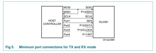
The device also supports full four-line SPI mode, the line SDIO serving as data input and P13/SDO as data output.
