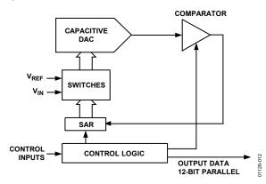
Figure 12. Simplified Block Diagram of AD7492
