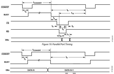
Figure 20. Parallel Port Timing with  $\overline{CS}$  and  $\overline{RD}$  Tied Low
