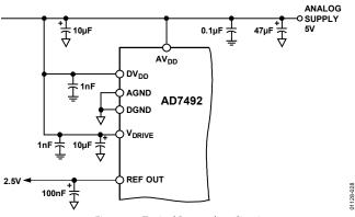
Figure 28. Typical Decoupling Circuit
