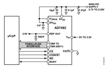
Figure 15. Typical Connection Diagram
