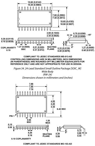
Figure 35. 24-Lead Thin Shrink Small Outline Package [TSSOP] (RU-24) Dimensions shown in millimeters
