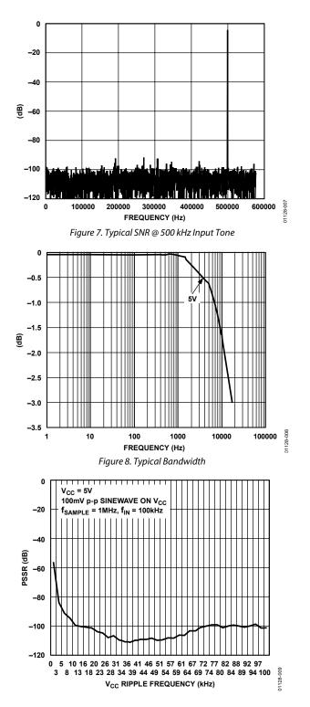
Figure 9. Typical Power Supply Rejection Ratio (PSRR)
