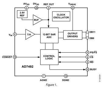
The type of sleep mode is hardware selected by the  $PS/\overline{FS}$  pin.
