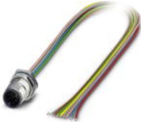
Sensor/actuator flush-type connector, 8-pos., M12 SPEEDCON, rear/screw mounting with M12 thread, with 0.5 m TPE litz wire, 8 x 0.25 mm
