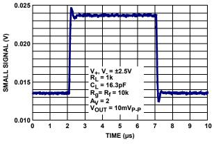
FIGURE 16. SMALL SIGNAL STEP RESPONSE
