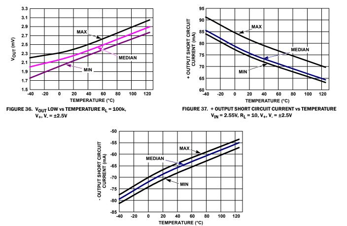
FIGURE 38. - OUTPUT SHORT CIRCUIT CURRENT vs TEMPERATURE V<sub>IN</sub> = -2.55V, R<sub>L</sub> = 10, V<sub>+</sub>, V<sub>-</sub> =  $\pm 2.5V$
