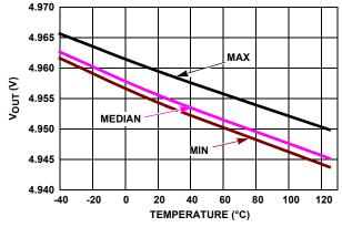
FIGURE 33.  $V_{OUT}$  HIGH vs TEMPERATURE R<sub>L</sub> = 1k,  $V_{+}, V_{-} = \pm 2.5V$
