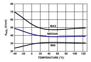
FIGURE 30. A<sub>VOL</sub> vs TEMPERATURE  $R_L = 1k$ ,  $V_+$ ,  $V_- = \pm 2.5V$ ,  $V_0 = -2V$ TO +2V
