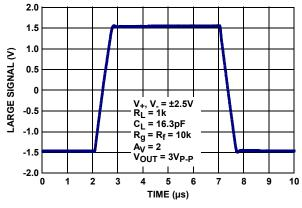
FIGURE 15. LARGE SIGNAL STEP RESPONSE
