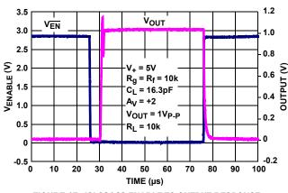
FIGURE 17. ISL28148 ENABLE TO OUTPUT RESPONSE
