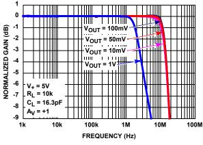
FIGURE 3. GAIN vs FREQUENCY vs  $V_{OUT}$ ,  $R_L = 10k$
