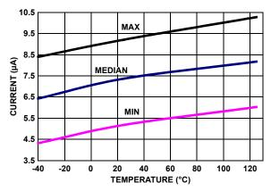
FIGURE 21. SUPPLY CURRENT DISABLED vs TEMPERATURE V<sub>+</sub>, V<sub>-</sub> =  $\pm 2.5V$
