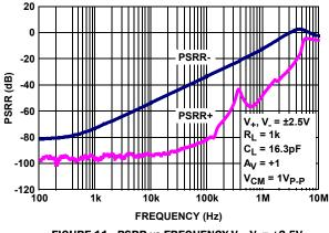
FIGURE 11. PSRR vs FREQUENCY V+, V\_ = ±2.5V
