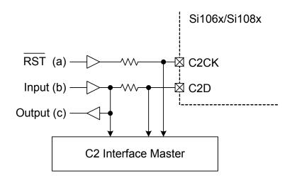
Figure 34.1. Typical C2 Pin Sharing
