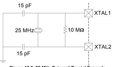
Figure 18.2. 25 MHz External Crystal Example
