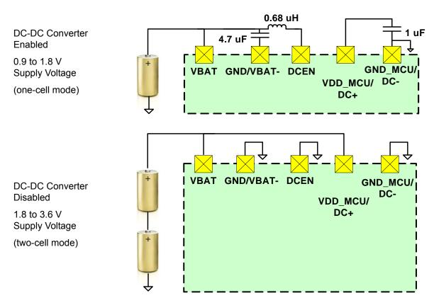
Figure 15.2. DC-DC Converter Configuration Options
