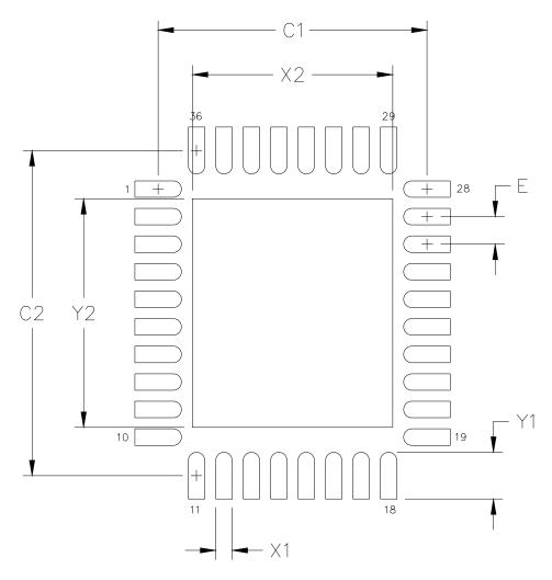
Figure 3.5. QFN-36 PCB Land Pattern Dimensions
