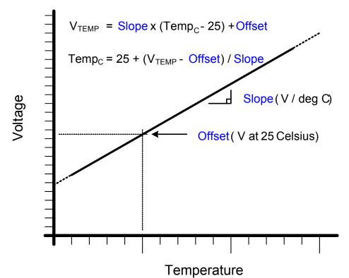
Figure 5.8. Temperature Sensor Transfer Function
