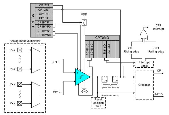
Figure 6.2. Comparator 1 Functional Block Diagram
