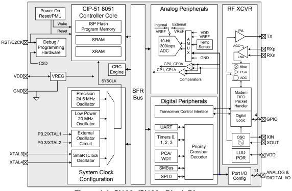
Figure 1.1. Si106x/Si108x Block Diagram
