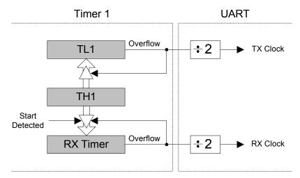
Figure 29.2. UART0 Baud Rate Logic
