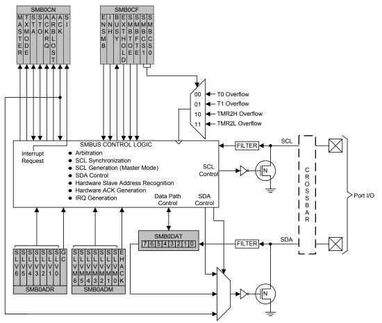
Figure 28.1. SMBus Block Diagram
