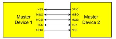
Figure 30.2. Multiple-Master Mode Connection Diagram
