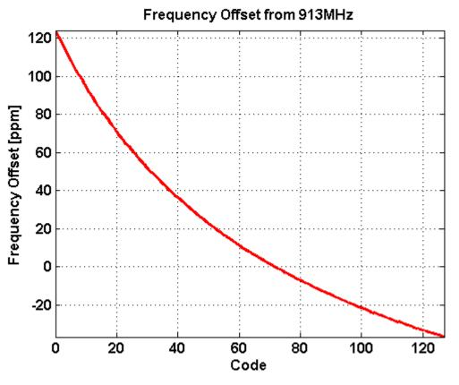
Figure 24.5. Capacitor Bank Frequency Offset Characteristics
