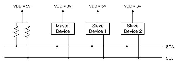
Figure 28.2. Typical SMBus Configuration
