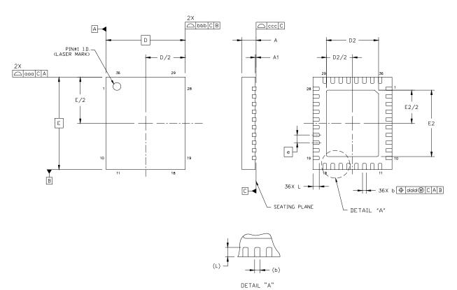
Figure 3.4. QFN-36 Package Drawing
