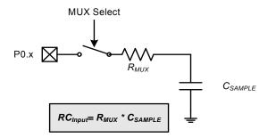
Note: The value of CSAMPLE depends on the PGA Gain. See Table 4.9 for details.
