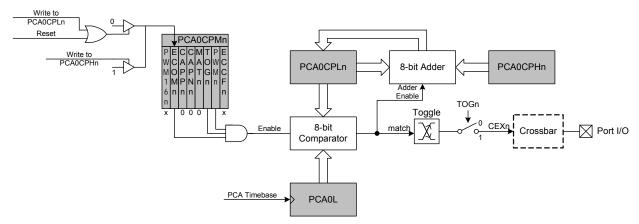
Figure 32.7. PCA Frequency Output Mode
