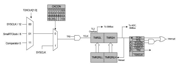
Figure 31.4. Timer 2 16-Bit Mode Block Diagram
