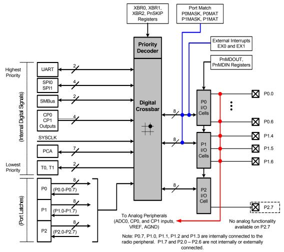
Figure 1.4. Port I/O Functional Block Diagram
