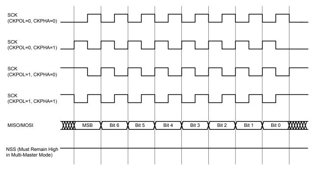
Figure 30.5. Master Mode Data/Clock Timing
