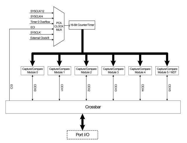
Figure 32.1. PCA Block Diagram
