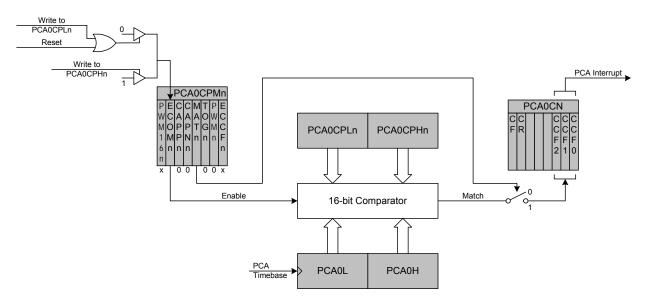
Figure 32.5. PCA Software Timer Mode Diagram
