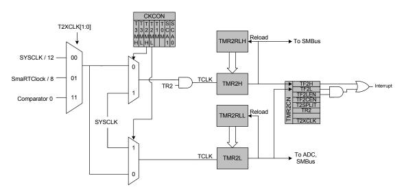
Figure 31.5. Timer 2 8-Bit Mode Block Diagram
