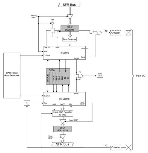
Figure 29.1. UART0 Block Diagram
