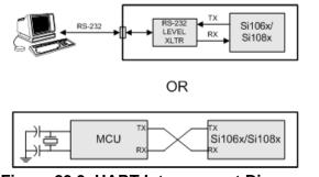
Figure 29.3. UART Interconnect Diagram
