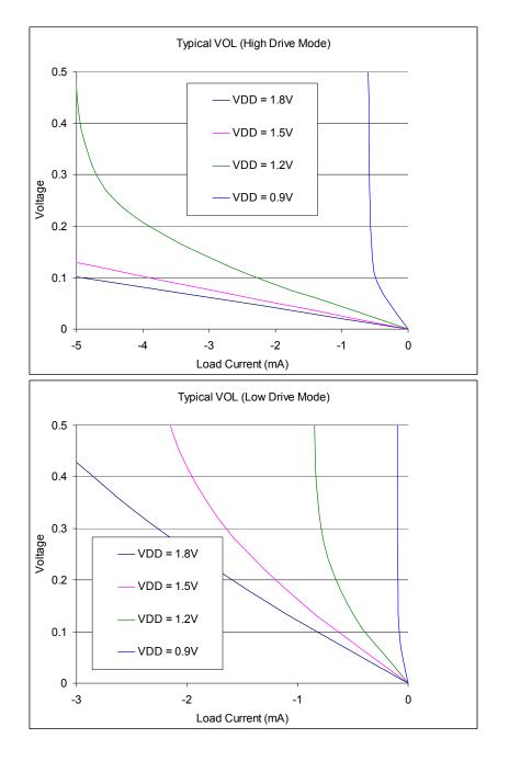
Figure 4.10. Typical VOL Curves, 0.9–1.8 V
