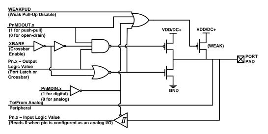
Figure 20.2. Port I/O Cell Block Diagram
