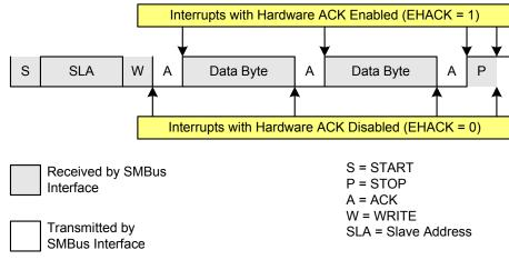
Figure 28.7. Typical Slave Write Sequence
