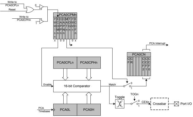
Figure 32.6. PCA High-Speed Output Mode Diagram
