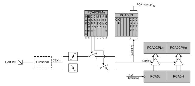
Figure 32.4. PCA Capture Mode Diagram
