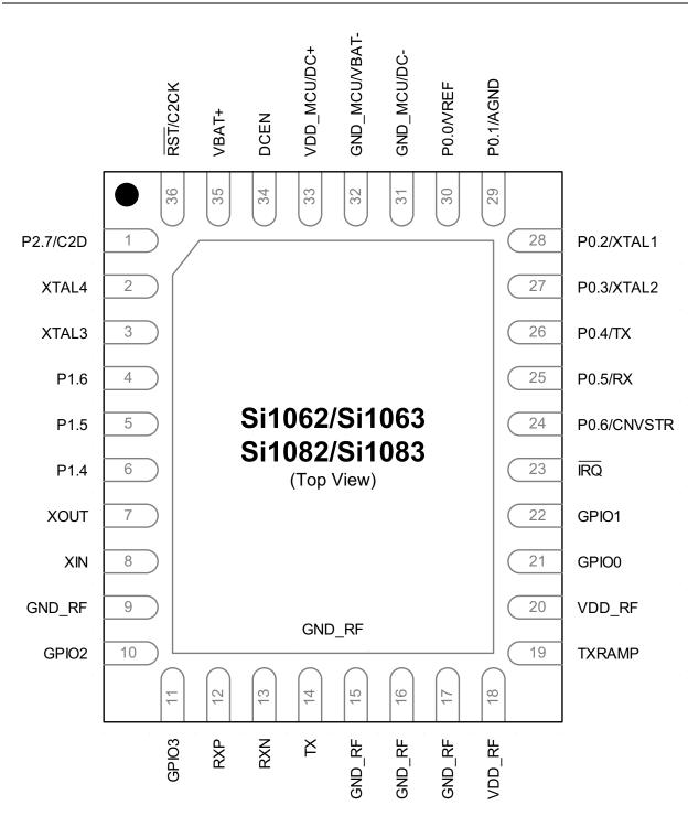
Figure 3.2. Si1062/3, Si1082/3-A-GM Pinout Diagram (Top View)
