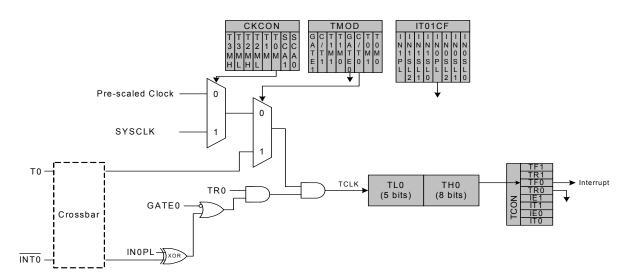
Figure 31.1. T0 Mode 0 Block Diagram
