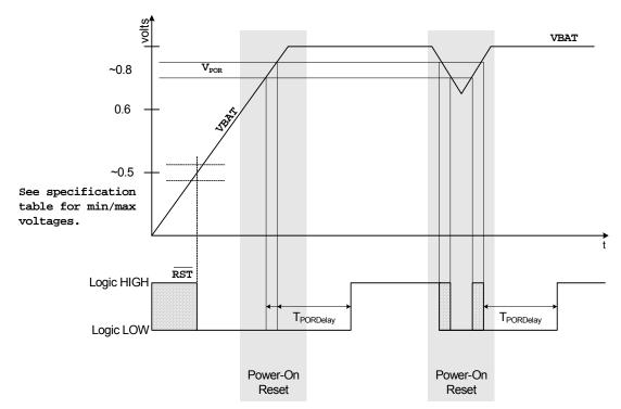
Figure 17.2. Power-Fail Reset Timing Diagram
