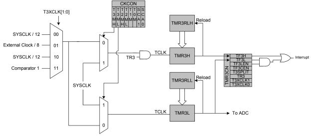
Figure 31.8. Timer 3 8-Bit Mode Block Diagram.
