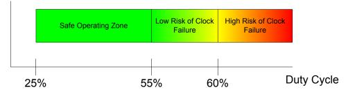
Figure 19.2. Interpreting Oscillation Robustness (Duty Cycle) Test Results
