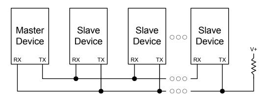
Figure 29.6. UART Multi-Processor Mode Interconnect Diagram
