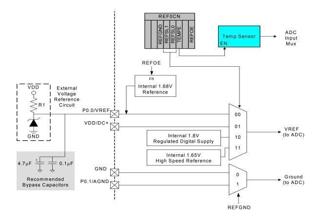
Figure 5.10. Voltage Reference Functional Block Diagram
