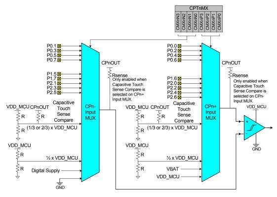
Figure 6.4. CPn Multiplexer Block Diagram
