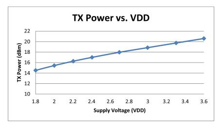
Figure 24.3. +20 dBm TX Power vs. VDD
