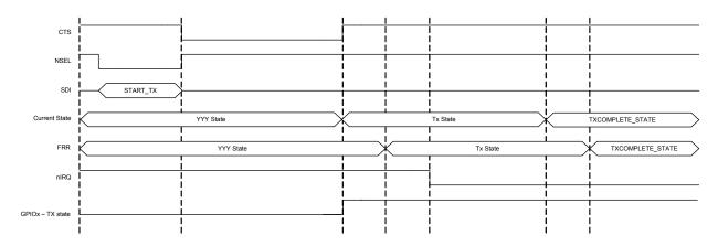
Figure 21.6. Start\_TX Commands and Timing
