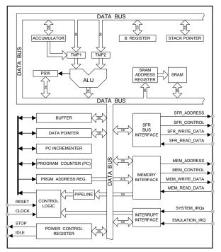
Figure 7.1. CIP-51 Block Diagram
