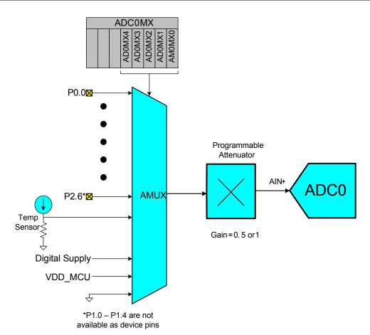
Figure 1.7. ADC0 Multiplexer Block Diagram
