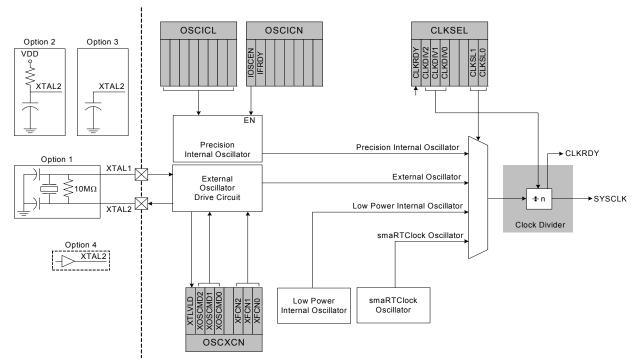
Figure 18.1. Clocking Sources Block Diagram
