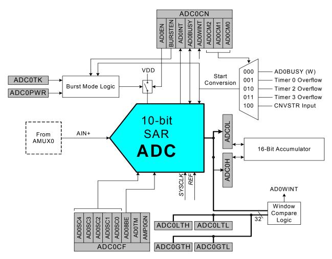
Figure 1.6. ADC0 Functional Block Diagram
