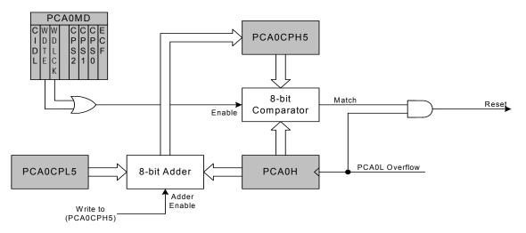
Figure 32.11. PCA Module 5 with Watchdog Timer Enabled
