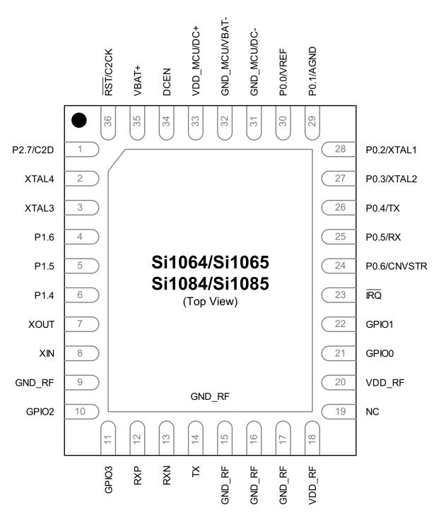
Figure 3.3. Si1064/5, Si1084/5-A-GM Pinout Diagram (Top View)
