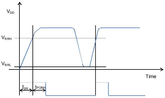
Figure 21.5. POR Timing Diagram
