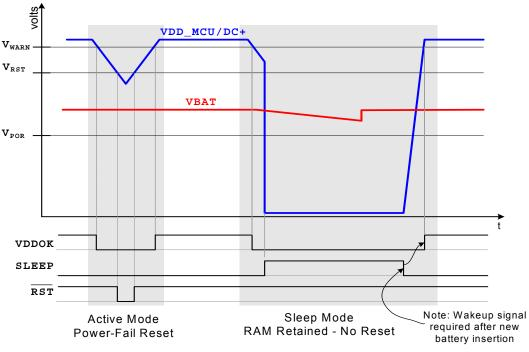
Figure 17.3. Power-Fail Reset Timing Diagram
