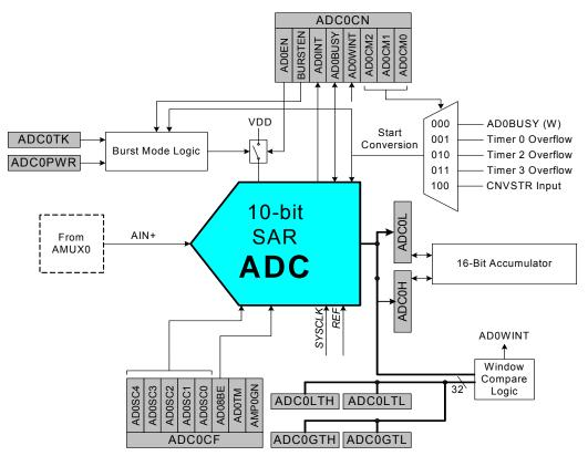
Figure 5.1. ADC0 Functional Block Diagram
