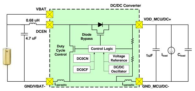
Figure 15.1. DC-DC Converter Block Diagram
