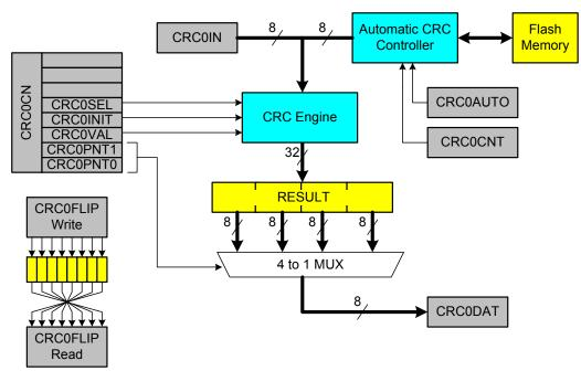
Figure 14.1. CRC0 Block Diagram
