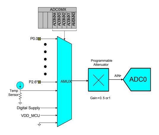
Figure 5.7. ADC0 Multiplexer Block Diagram
