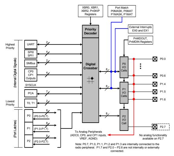
Figure 20.1. Port I/O Functional Block Diagram
