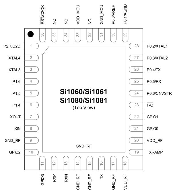
Figure 3.1. Si1060/1, Si1080/1-A-GM Pinout Diagram (Top View)
