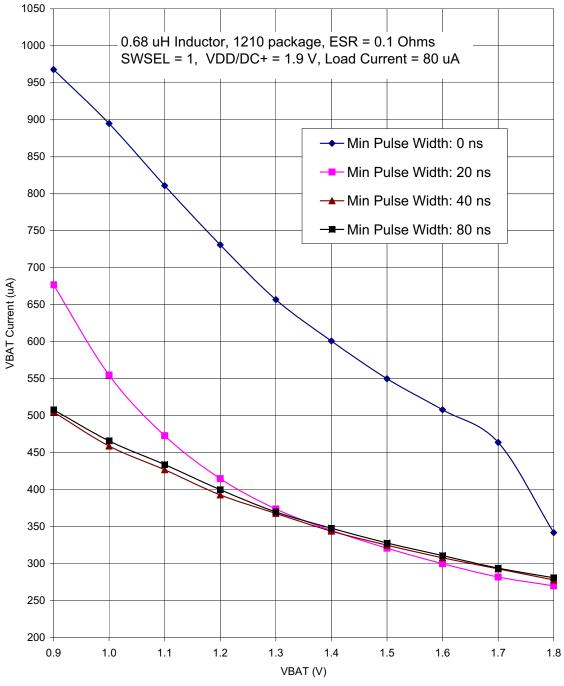
Figure 4.6. Typical One-Cell Suspend Mode Current
