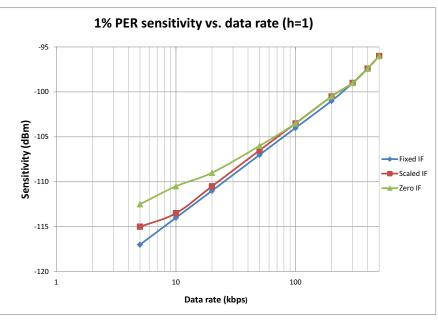
Figure 24.1. RX Architecture vs. Data Rate
