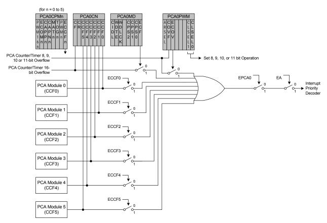
Figure 32.3. PCA Interrupt Block Diagram
