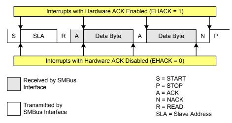
Figure 28.6. Typical Master Read Sequence
