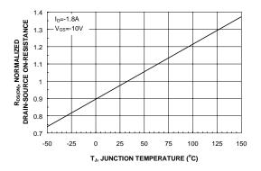
Figure 3. On-Resistance Variation with Temperature.
