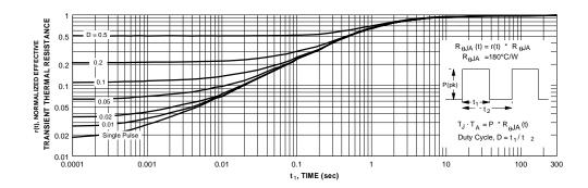
Figure 11. Transient Thermal Response Curve.
