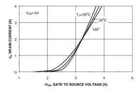
Figure 5. Transfer Characteristics.
