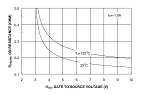
Figure 4. On-Resistance Variation with Gate-to-Source Voltage.
