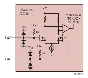
Figure 8a. Equivalent Encode Input Circuit
