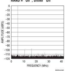
$$\label{eq:local_local_local_local} \begin{split} LTC2206\text{-}14\text{: }32\text{K Point FFT, }f_{IN} \\ = 14\text{.}86\text{MHz, }-1\text{dBFS, PGA} = 0, \\ RAND = "On", Dither "Off" \end{split}$$
