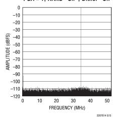
LTC2207-14: 32K Point 2-Tone FFT,  $f_{IN} = 69.2MHz$  and 76.5MHz, -7dBFS, PGA = 0, RAND "On", Dither "Off"
