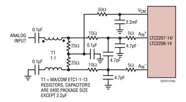
Figure 4a. Using a Transmission Line Balun Transformer.
