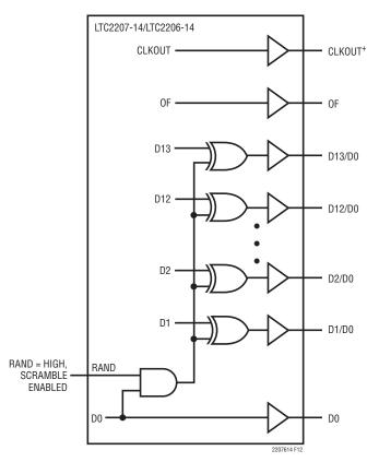
Figure 12. Functional Equivalent of Digital Output Randomizer
