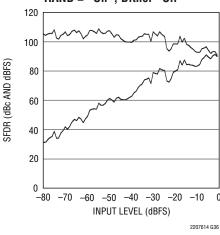
LTC2206-14: SFDR vs Input Level, f<sub>IN</sub> = 15.1MHz, PGA = 0, RAND = "0n", Dither "0n"
