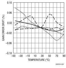
Gain Error Drift vs Temperature, Internal Reference, 5 Units Drift from 25°C
