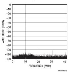
LTC2206-14: 32K Point FFT,  $f_{\text{IN}}$  = 70.24MHz, -1dBFS, PGA = 1, RAND = "On", Dither "Off"
