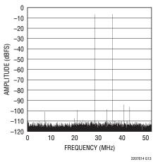
LTC2207-14: 32K Point 2-Tone FFT, f<sub>IN</sub> = 69.2 MHz and 76.5 MHz, -15 dBFS,PGA = 0, RAND "On", Dither "Off"
