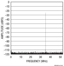
LTC2207-14: 64K Point FFT,  $f_{IN} = 70.1MHz, -25dBFS$ PGA = 0, RAND "On", Dither "On'
