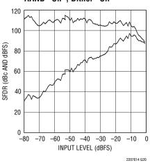
LTC2207-14: SFDR vs Input Level,  $f_{IN} = 140.1MHz$ , PGA = 1, RAND "On", Dither "On"
