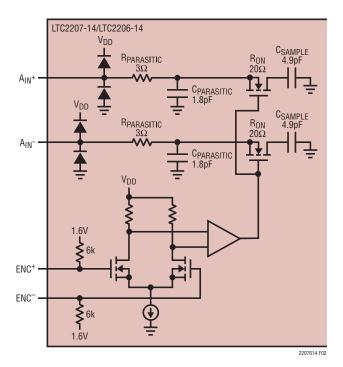
Figure 2. Equivalent Input Circuit
