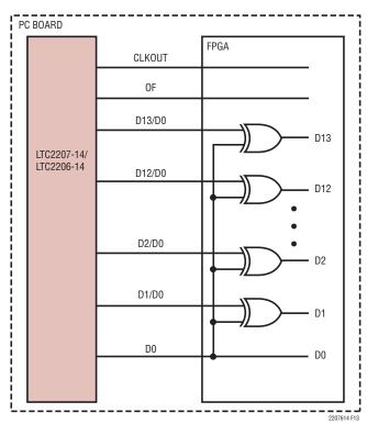
Figure 13. Descrambling a Scrambled Digital Output
