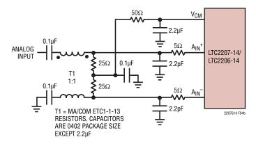
Figure 4b. Using a Transmission Line Balun Transformer.
