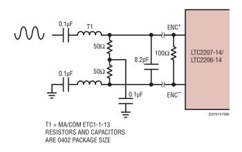
Figure 8b. Transformer Driven Encode
