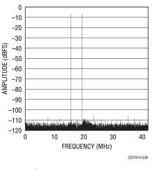
LTC2206-14: 32K Point 2-Tone FFT, f<sub>IN</sub> = 14.87MHz and 18.56MHz, -15dBFS, PGA = 0, RAND = "On", Dither "Off"
