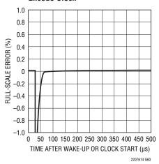
Full-Scale Settling After Wake Up from Shutdown or Starting Encode Clock
