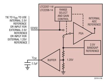
Figure 6. Reference Circuit
