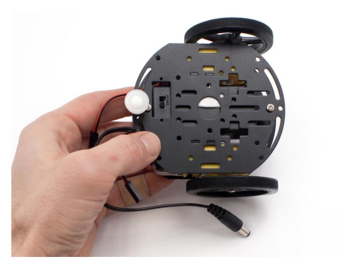
Place the battery box back in between the motors and stick it to the chassis
