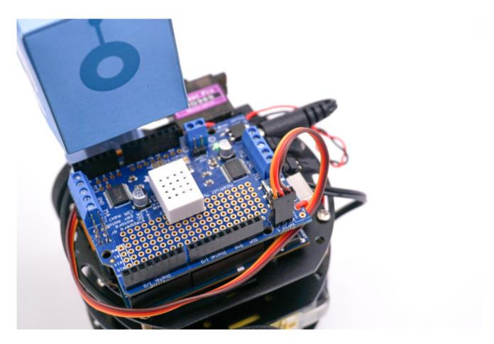
Open the **Ada\_CurieBot\_RC\_CandyServo** sketch in the Arduino IDE, and then upload it to CurieBot.
