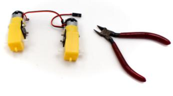
To make space for the 9V battery pack later, trim the excess off of the inner motor wheel shaft on each motor. Grab some diagonal cutters (scissors or a hobby knife will work in a pinch) and trim off about half the length of the motor wheel shaft that is on the same side as the black plate you affixed.
