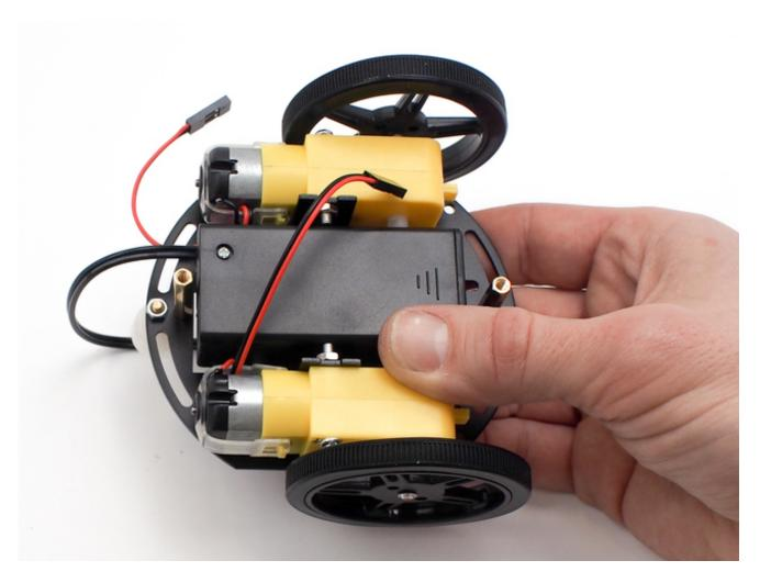
Check to see that the 9V box fits between the motors -- trim more of the inner shafts if needed.
