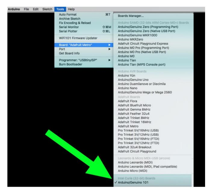
In case you don't see that board choice, you can click on Arduino IDE Tools > Board > Boards Manager... and then sort the list in the Boards Manager search bar with the word "101" and then update the AVR boards definition and install the 101 board as seen here.
