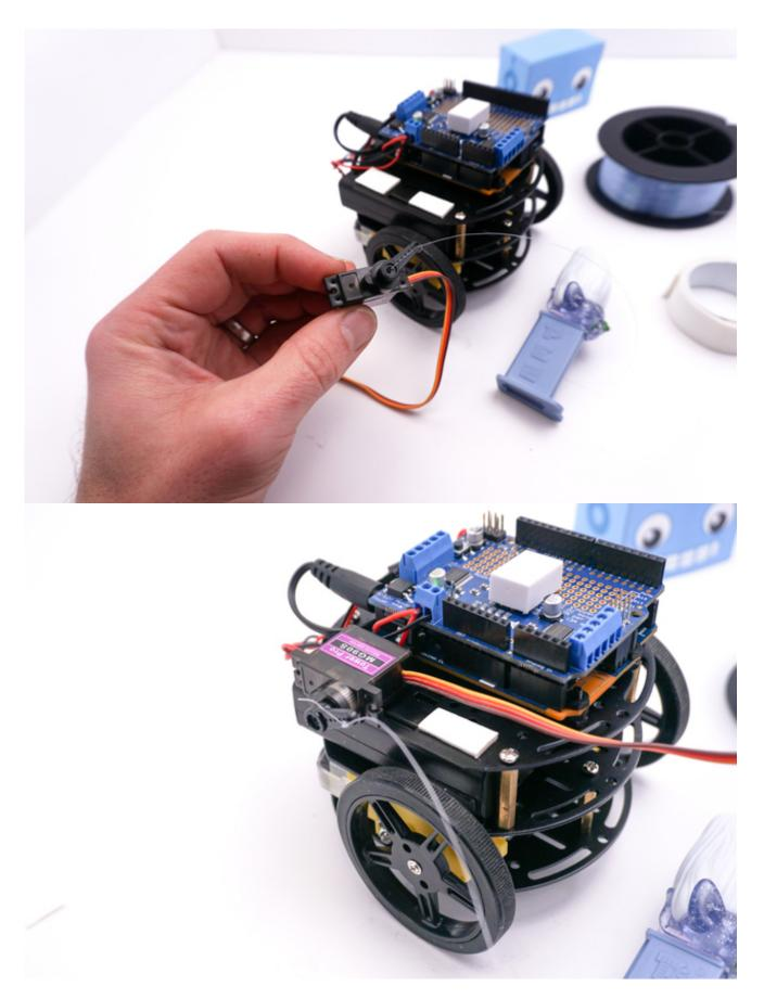
Tie the filament to the dispenser's head so the line is taut when the servo is at its resting
