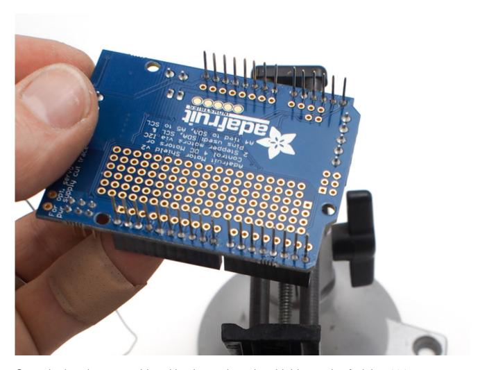
Once the headers are soldered in place, place the shield onto the Arduino 101.
