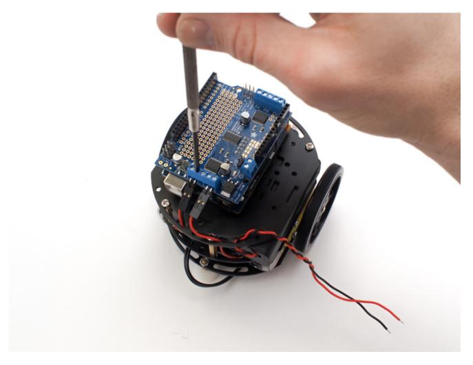
Make sure the battery packs are both turned off, then plug the 9V barrel plug into the jack on the Arduino 101.
