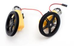
Fit the wheels onto the white knob on the motors, they will snap nicely onto the oval center.
