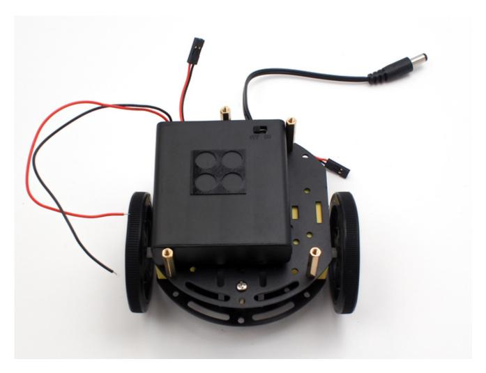
Notice the battery box is lined up on the left side of the middle chassis plate. It should be just in-between the upper left stand-off and the lower left stand-off (not touching either). This will make sure the on-off switch lines up just right in the hole of the top plate.
