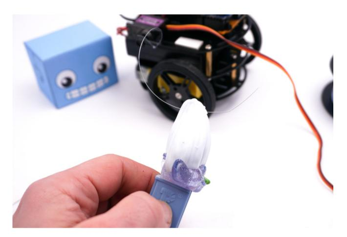
Use a couple of pieces of double stick foam tape to mount the micro servo and candy dispenser to the top plate of CurieBot. You can also drill a small hole into the foot of the candy dispenser base and screw it in place on one of the robot's brass standoffs.
