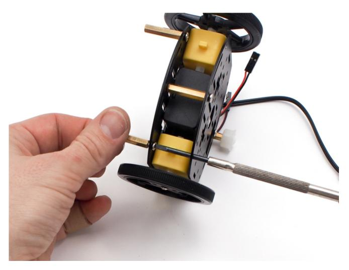
Take a look at the image below and install the brass stand-offs in the same positions. You can insert the stand-off screws through the middle plate and hand tighten the stand-offs while putting a bit of pressure on the screw with your finger. Or, as a tip, you can screw in the stand-off screws with the flat end of the screwdriver, which can reach through the holes in the bottom plate.
