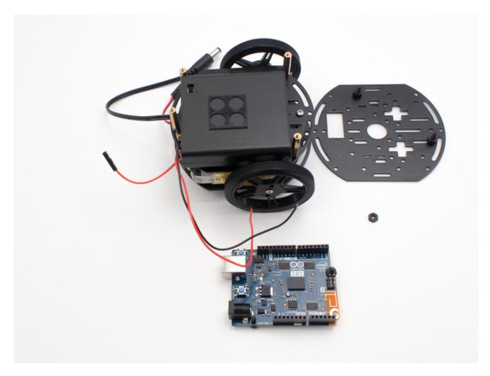
Screw in the two screws and four nuts that'll protrude from the top of the middle chassis layer as seen below, then place the layer on top of the AA battery box.
