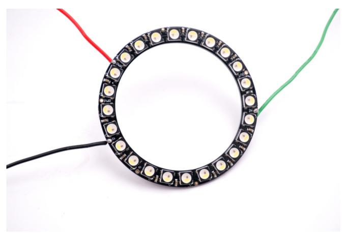
Solder leads to the **DIN**, **+5V**, and **GND** pins on the NeoPixel ring. Solid core hookup wire is a nice choice, as it can serve double duty as the structural connection to hold the ring in place underneath.
