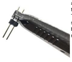
For this next step, you will need a set of pliers. First, grab the long header pins that are attached together and break them into 2 sets of 2 header pins. Then, grab them in the pliers like shown here, and then slightly bend them so they look like the next picture.
