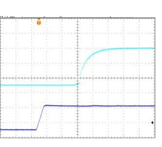
*Figure 6:* Turn-on transient at zero load current (10 ms/div). Top Trace: Vout; 2V/div; Bottom Trace: input voltage: 30V/div.
