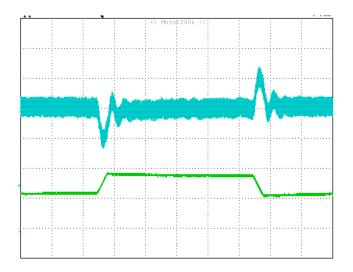
**Figure 8:** Output voltage response to step-change in load current (50%-75%-50% of full load; di/dt =  $0.1A/\mu$ s).
