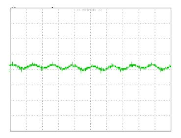
**Figure 12:** Input reflected ripple current,  $i_s$ , through a  $12\mu$ H source inductor at nominal input voltage and max load current (10 mA/div, 2us/div).
