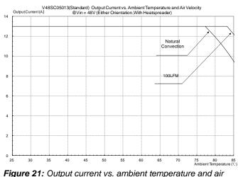
velocity @Vin=48V(Either Orientation, with heat spreader)
