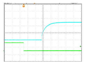
*Figure 5:* Turn-on transient at full load current (10 ms/div). Top Trace: Vout: 2V/div; Bottom Trace: ON/OFF input: 5V/div.
