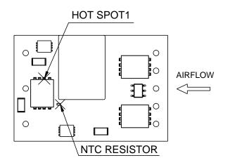
Figure 18: \* Hot spot 1& NTC resistor temperature measured points, the allowed maximum hot spot 1 temperature is defined at 122  ${}^\circ\!\!C$
