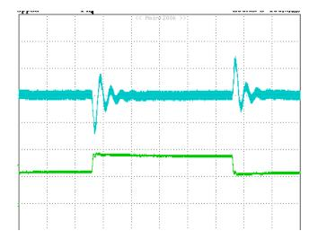
**Figure 9:** Output voltage response to step-change in load current (50%-75%-50% of full load; di/dt =  $2.5A/\mu$ s). Load cap:  $10\mu$ F, tantalum capacitor and  $1\mu$ F ceramic capacitor. Top Trace: Vout; 200mV/div; Bottom Trace: output current: 5A/div, Time: 100us/div
