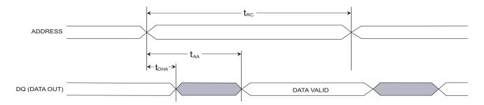
Figure 6. SRAM Read Cycle 2:  $\overline{\text{CE}}$  and  $\overline{\text{OE}}$  Controlled <sup>[5]</sup>
