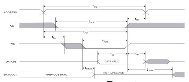
Figure 8. SRAM Write Cycle 2: CE Controlled [9]
