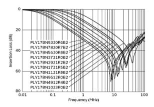
Common Mode Insertion Loss-Frequency Characteristics
