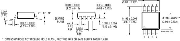
PROTRUSIONS OR GATE BURRS SHALL NOT EXCEED 0.006" (0.152mm) PER SIDE \*\* DIMENSION DOES NOT INCLUDE INTERLEAD FLASH OR PROTRUSIONS.
