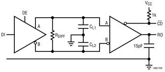
Figure 4. Driver/Receiver Timing Test Load
