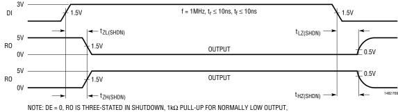
NOTE: DE = 0, RO IS THREE-STATED IN SHUTDOWN, 1k $\Omega$  PULL-UP FOR NORMALLY LOW OUTPUT, 1k $\Omega$  PULL-DOWN FOR NORMALLY HIGH OUTPUT
