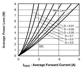
Fig. 6 - Forward Power Loss Characteristics
