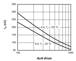
Fig. 7 - Typical Reverse Recovery Time vs. dl<sub>F</sub>/dt
