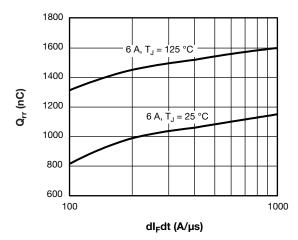
Fig. 8 - Typical Stored Charge vs. dl<sub>F</sub>/dt
