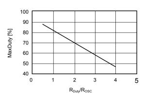
Figure 13 R<sub>Duty</sub>/R<sub>OSC</sub> vs. MaxDuty
