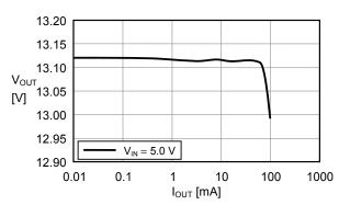
(2) fosc = 700 kHz, MaxDuty = 77 % (Rosc = 200 k $\Omega$ , R<sub>Duty</sub> = 300 k $\Omega$ )
