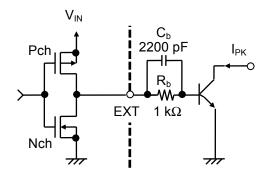
Figure 11 External Transistor Periphery
