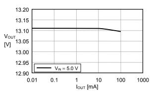
(3) fosc = 286 kHz, MaxDuty = 77 % (Rosc = 510 k $\Omega$ , R<sub>Duty</sub> = 750 k $\Omega$ )
