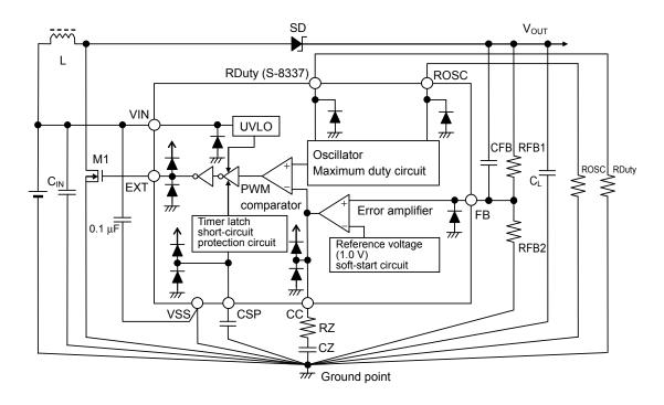
Figure 15 Standard Circuit (S-8337 Series)
