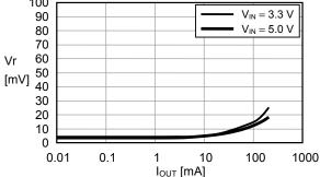
(3) fosc = 286 kHz, MaxDuty = 77 % (Rosc = 510 k $\Omega$ , R<sub>Duty</sub> = 750 k $\Omega$ )
