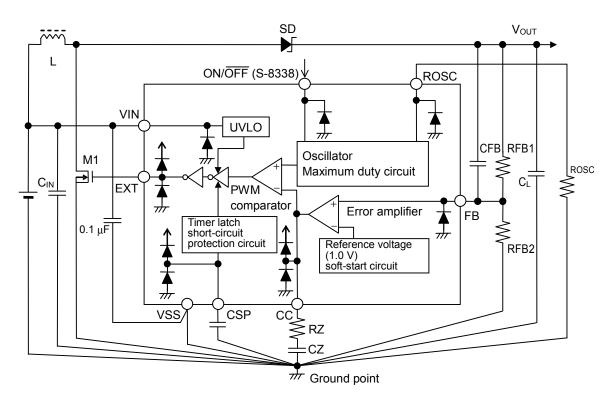
Figure 16 Standard Circuit (S-8338 Series)
