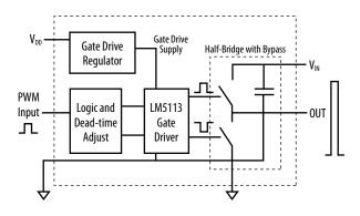
Figure 1: Block Diagram of EPC9001 Development Board
