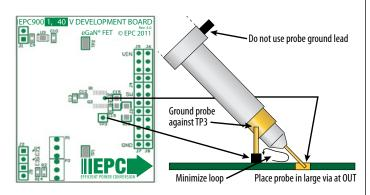
Figure 3: Proper Measurement of Switch Node — OUT
