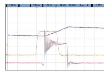
Figure 4: Typical Waveforms for V<sub>IN</sub> = 24 V to 1.2 V/15 A (500kHz) Buck converter CH1: V<sub>PWM</sub> Input voltage – CH3: (lour) Switch node current – CH4: (Vour) Switch node voltage
