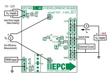
Figure 2: Proper Connection and Measurement Setup
