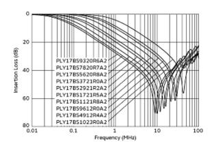
Common Mode Insertion Loss-Frequency Characteristics
