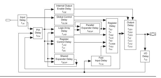
The timing characteristics of any signal path can be derived from the timing model and parameters of a particular device. External timing parameters, which represent pin-to-pin timing delays, can be calculated as the sum of internal parameters. Figure 12 shows the timing relationship between internal and external delay parameters.
