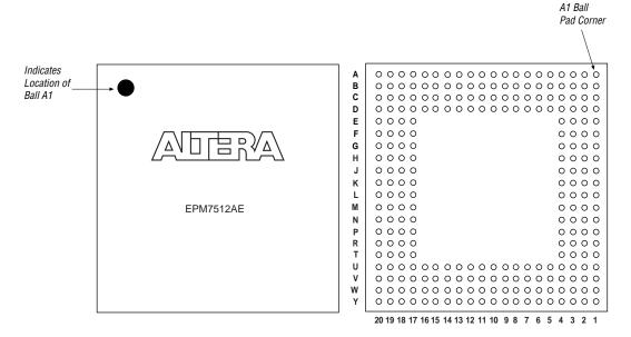
Figure 23. 256-Pin FineLine BGA Package Pin-Out Diagram
