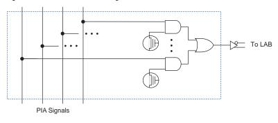
While the routing delays of channel-based routing schemes in masked or FPGAs are cumulative, variable, and path-dependent, the MAX 7000A PIA has a predictable delay. The PIA makes a design's timing performance easy to predict.
