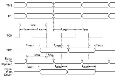
Figure 8. MAX 7000A JTAG Waveforms
