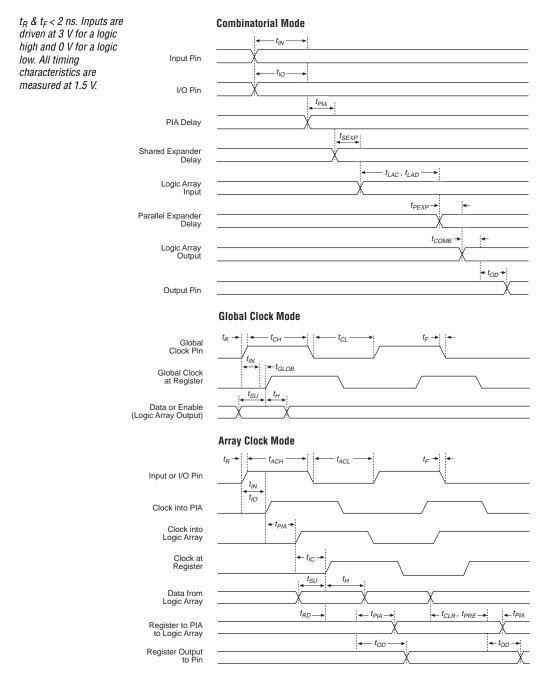
Tables 17 through 30 show EPM7032AE, EPM7064AE, EPM7128AE, EPM7256AE, EPM7512AE, EPM7128A, and EPM7256A timing information.
