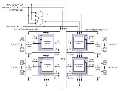
Figure 1. MAX 7000A Device Block Diagram
