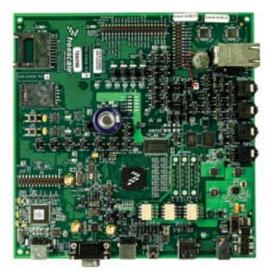
The MCF5301x family of 32-bit MCUs combines low power, high integration and extensive connectivity with an audio subsystem, into a powerful platform for general industrial control applications, including digital voice functionality for intercom and public address systems.The audio system includes a speech codec, microphone, headset and loud speaker amplifiers, and an optional NRE-free VoIP-based digital voice solution designed specifically for industrial and consumer applications.
