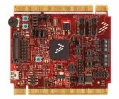
The 32-bit dual-core PXN20 Power Architecture MCU supports a variety of communication protocols, allowing you to design a cost-effective, reliable industrial gateway with cutting-edge performance. A large amount of on-chip flash, on-chip SRAM with error correction code capability, 36-channel ADC, dual cores and a host of serial I/Os make the PXN20 a compelling solution for your next design cycle.
