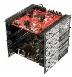
MCF51EM256 is Freescale's new smart-meteron-a-chip 32-bit ColdFire V1 core MCU with embedded LCD controller, 16-bit ADC and metrology-specific peripherals optimized for smart meter applications. MCF51EM256 comes with a full suite of hardware and software tools to make development quick and easy.
