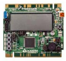
Freescale expands the first S08 ultra-low-power MCU with LCD driver and increased ADC accuracy for medical and metering applications. The MC9S08LH family available with up to 64 KB flash helps you reach your target performance levels while minimizing power consumption in your design, demonstrating extreme energy efficiency for ultra-long operation in battery-powered applications. The S08LH also features a 16-bit ADC for accurate measurement.
