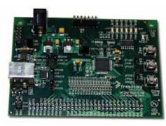
The MC56F802x/3x family combines the processing power of a DSP with the functionality and ease of use of an MCU on a single chip. With a flexible set of peripherals, package and memory options from 16 to 64 KB flash memory, CAN and high-resolution PWM/timers running at up to 96 MHz, the 56F8000 series provides a cost-effective high-performance solution.
