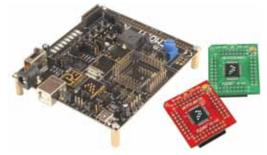
With 8- and 32-bit compatibility, as well as compatibility within our USB MCU portfolio, the JM family offers exceptional migration flexibility. The S08JM family of MCUs provides a completely integrated USB solution with a complimentary USB stack to make development quick and easy while expanding our low-end USB portfolio. The MC9S08JS offers smaller package options to optimize cost in USB-enabled designs. The MC9S08JS also featured a pre-loaded USB bootloader.
