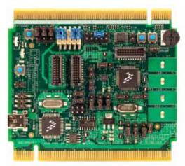
The PXS devices are 32-bit Power Architecture embedded MCUs designed for safety critical applications. All devices in this family are built around a dual core safety architecture and offer more processing power and larger memory sizes to handle a variety of industrial designs. The dualcore can be operated in lockstep mode (redundant processing and calculations) or decoupled parallel mode (independent core operations). The PXS MCUs are SafeAssure solutions.
