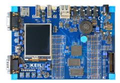
The Keil MCB4300 Evaluation Board enables you to create and test working programs based on the NXP LPC4300 family of ARM Cortex<sup>™</sup>-M4 processor-based devices.
