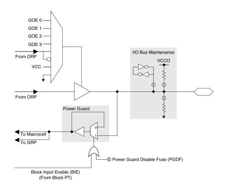
Each output supports a variety of output standards dependent on the  $V_{CCO}$  supplied to its I/O bank. Outputs can also be configured for open drain operation. Each input can be programmed to support a variety of standards, independent of the  $V_{CCO}$  supplied to its I/O bank. The I/O standards supported are:
