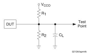
Table 13. Test Fixture Required Components
